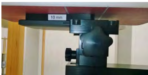
Photo of the device positioned for WR mode measurement – display facing phantom. The spacer was removed before the start of the measurements.
