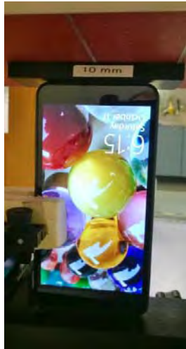
Photo of the device positioned for WR mode measurement – bottom edge facing phantom. The spacer was removed before the start of the measurements.
