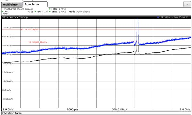
Note: The peak above the limit is the carrier frequency. This plot is valid for Chain A, Chain B, Chain A+B.
