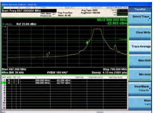
LTE Band 12 16QAM 1.4MHz CH-High, 1 RB 716MHz~717MHz
