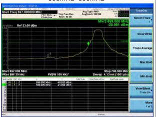
LTE Band 12 QPSK 3MHz CH-High, 1 RB 716MHz~717MHz
