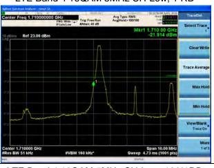
LTE Band 4 16QAM 5MHz CH-High, 1 RB
