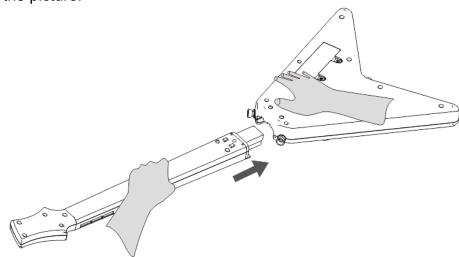
After the piano rod is connected, fix the two screws in the position shown below to prevent the piano rod from coming out.
