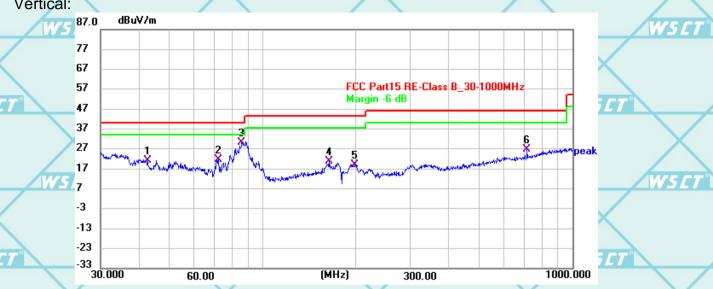
Frequency Reading Factor Level Limit Margin No. Detector (MHz) (dBuV) (dB/m) (dBuV/m) (dBuV/m) (dB) 1 42.7121 40.11 -18.8521.26 40.00 -18.74QP 2 72.1476 44.36 -22.62 21.74 40.00 -18.26QP 3 \* 85.7854 54.27 -23.91 30.36 40.00 -9.64 QP 40.78 20.82 43.50 -22.68 QP 4 163.8267 -19.965 19.07 QP 198.8493 42.86 -23.7943.50 -24.43 QΡ 6 714,1734 38.67 -12.0726.60 46.00 -19.40
