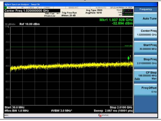
Antenna 1 / (2 Port) 5G NR n66 25 MHz 1 Carrier + LTE B66 5 MHz 1 Carrier [2 Carrier] / Low Edge-100 ~ Low Edge / 16QAM / Non-Contiguous
