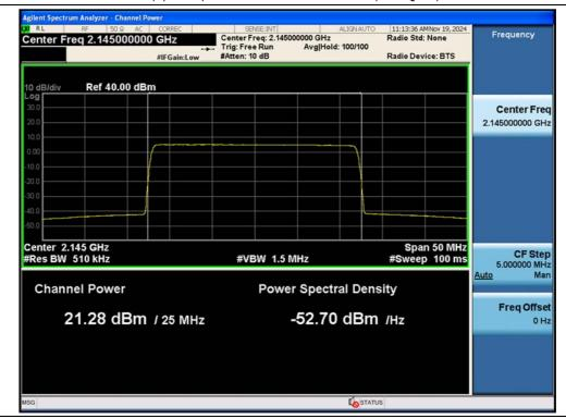
Antenna 1 / (2 Port) 5G NR n66 25 MHz 1 Carrier / 256QAM / Middle
