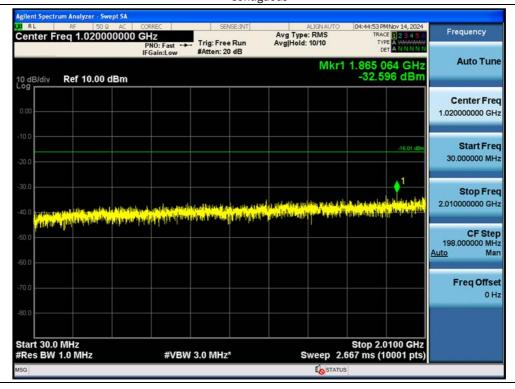
Antenna 1 / (2 Port) 5G NR n66 25 MHz 1 Carrier + LTE B66 5 MHz 1 Carrier [2 Carrier] / Low Edge-100 ~ Low Edge / 64QAM / Low / Contiguous
