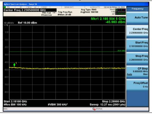
Antenna 1 / (2 Port) 5G NR n66 25 MHz 1 Carrier + 5G NR n66 5 MHz 1 Carrier [2 Carrier] / High Edge+100 ~ 10 GHz / 256QAM / Non-Contiguous
