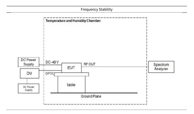
**Note:** All modulations(QPSK, 16QAM, 64QAM, 256QAM) were investigated and the worst case configuration channel results are reported.
