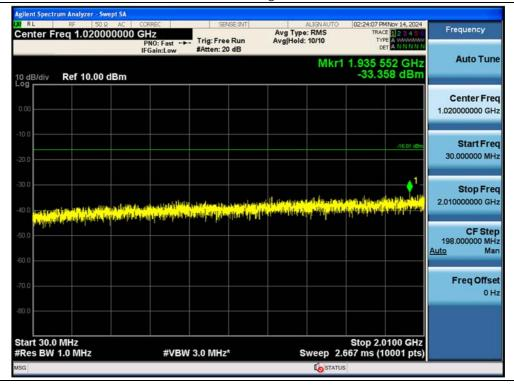
Antenna 1 / (2 Port) 5G NR n66 25 MHz 1 Carrier + 5G NR n66 5 MHz 1 Carrier [2 Carrier] / Low Edge-100 ~ Low Edge / 16QAM / Non-Contiguous
