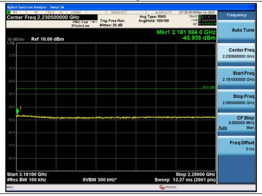
Antenna 1 / (2 Port) 5G NR n66 25 MHz 1 Carrier + LTE B66 5 MHz 1 Carrier [2 Carrier] / High Edge+100 ~ 10 GHz / 64QAM / Non-Contiguous
