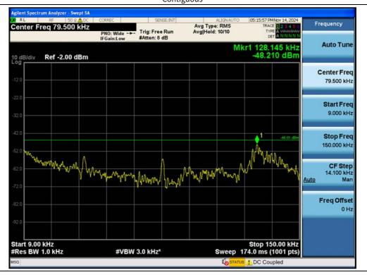
Antenna 1 / (2 Port) 5G NR n66 25 MHz 1 Carrier + LTE B66 5 MHz 1 Carrier [2 Carrier] / 150 kHz ~ 30 MHz / 256QAM / Middle / Contiguous
