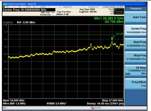
Antenna 0 / (2 Port) 5G NR n66 25 MHz 1 Carrier / 10 GHz ~ 26.5 GHz / QPSK / High
