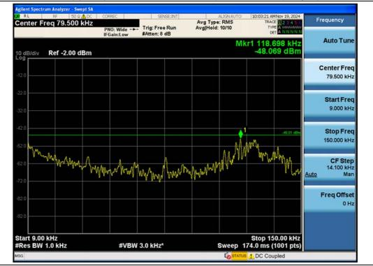
Antenna 1 / (2 Port) 5G NR n66 25 MHz 1 Carrier / 9 kHz ~ 150 kHz / 16QAM / Low
