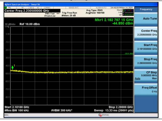
Antenna 1 / (2 Port) 5G NR n66 25 MHz 1 Carrier + LTE B66 5 MHz 1 Carrier [2 Carrier] / High Edge+100 ~ 10 GHz / 64QAM / High / Contiguous
