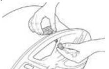
Screw the nut onto the sensor valve by hand.
