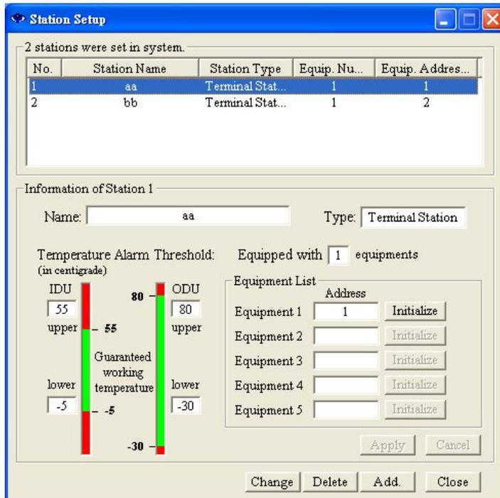
Figure 8-18: Temperature Alarm Threshold
