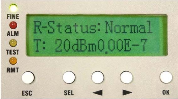
Figure 5-47 R-Status:Test/Normal
