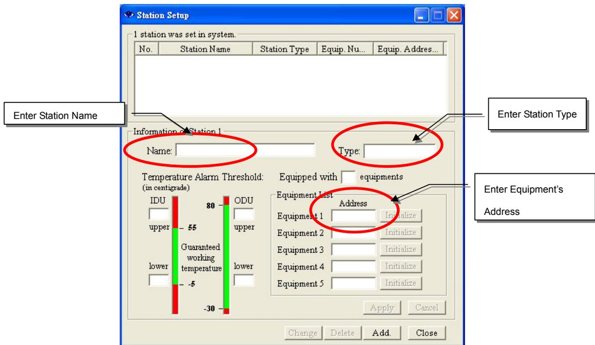
Figure 8-14: Station Setup (1)
