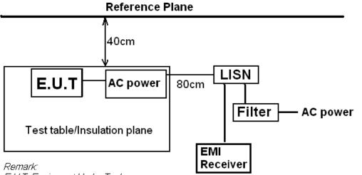
E.U.T: Equipment Under Test LISN: Line Impedence Stabilization Network Test table height=0.8m
