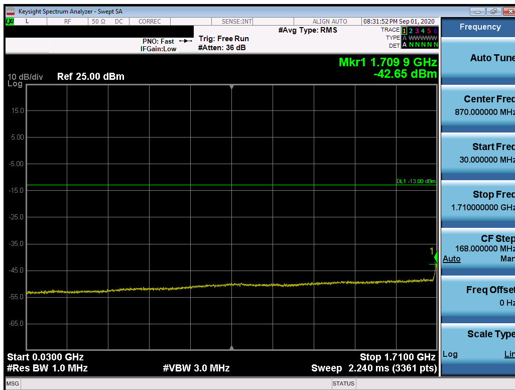
Plot 7-120. Conducted Spurious Plot (LTE Band 66/4 - 20MHz QPSK - RB Size 1, RB Offset 0 - Mid Channel)
