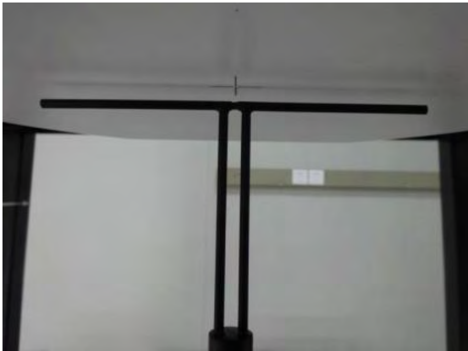
Photo of Dipole Setup
