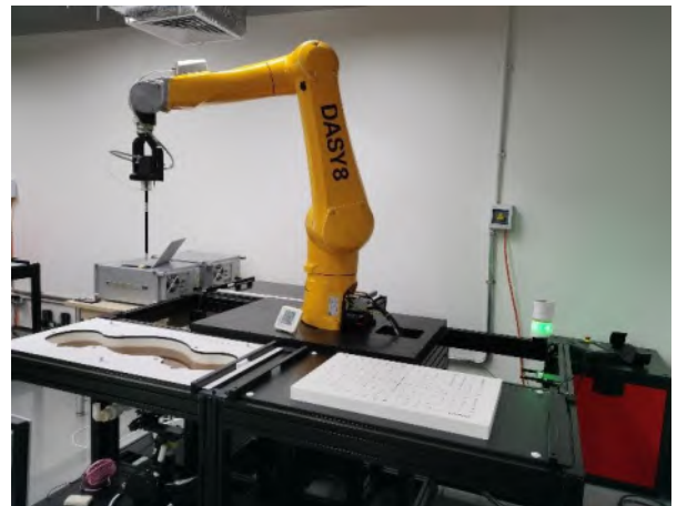
Picture D.6 Specific Absorption Rate Test Layout
