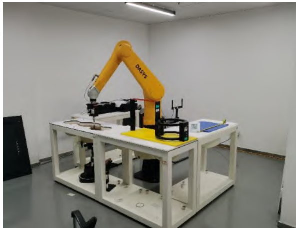
Picture D.6 Specific Absorption Rate Test Layout
