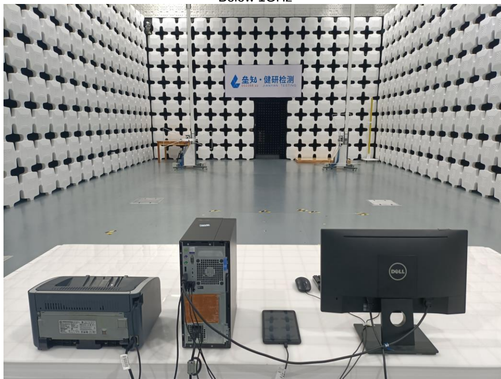
Radiated Emission Below 1GHz
