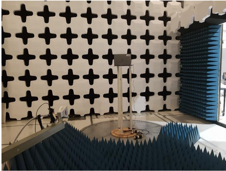
Photograph 3. Radiated Cabinet Spurious Emissions Test Setup, 18-25 GHz
