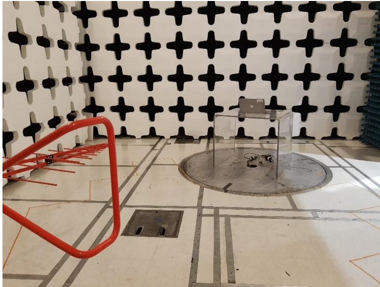
Photograph 1. Radiated Cabinet Spurious Emissions Test Setup, 30-1000MHz
