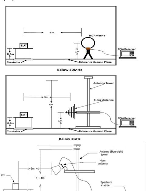
Above 18 GHz shall be extrapolated to the specified distance using an extrapolation factor of 20 dB/decade form 3m to 1m.
