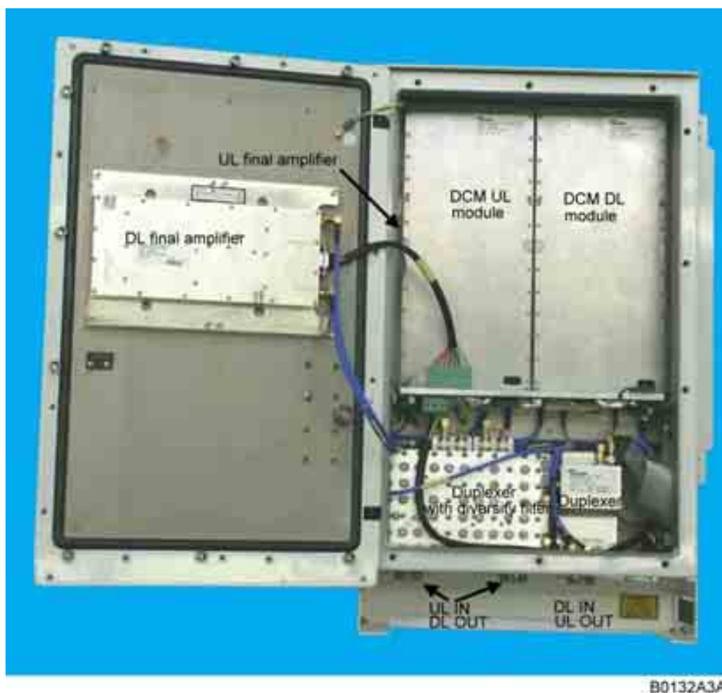
figure 5-3 RF path of a Node C, exemplary
