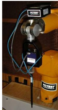
Figure 9 SPEAG Robotic System
