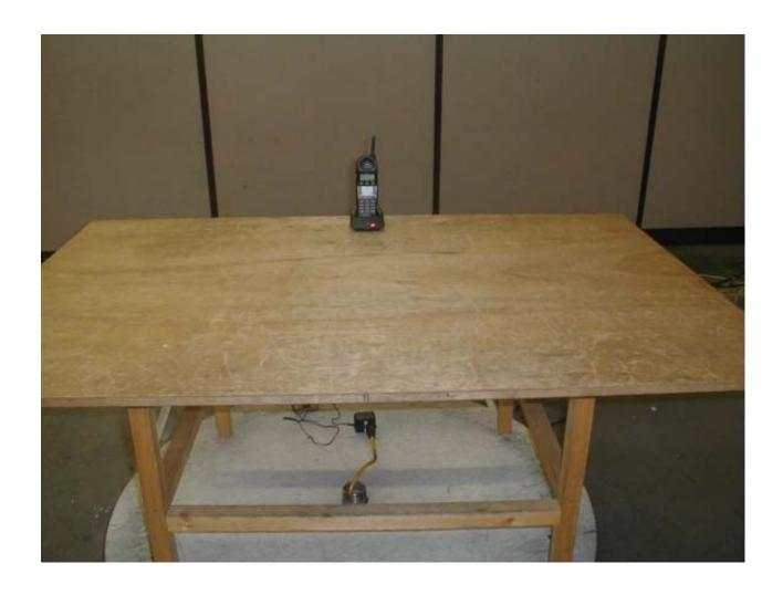
**EUT – Handset Radiation Setup Test Rear View**
