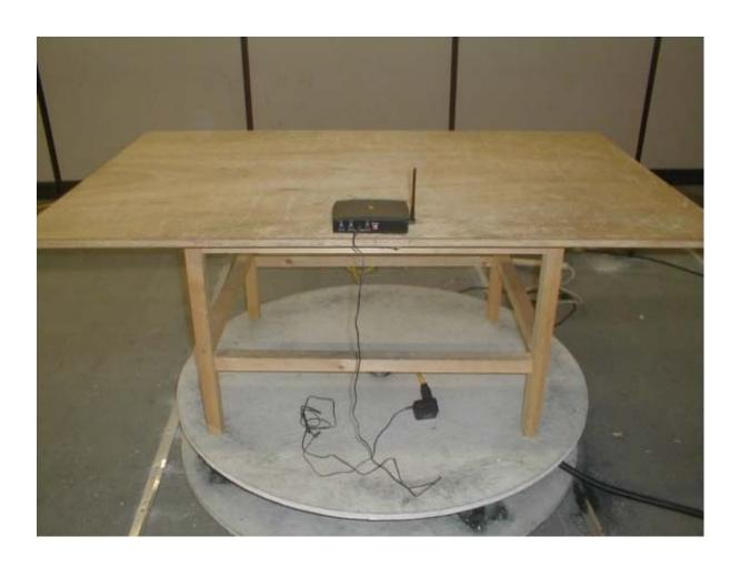
**EUT - Handset Radiation Setup Test Setup**
