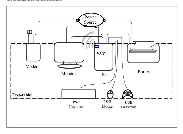
The tests below are carried with the EUT transmitter set at high power in TDD mode. The EUT is forced to select of output power level and channel number by PC.
