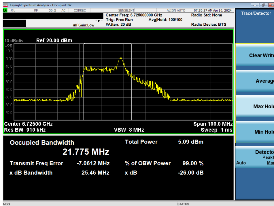
Plot 7-12. Occupied Bandwidth Plot MIMO ANT1 (40MHz BW 802. 11be (26 Tones) (UNII Band 7) – Ch. 155)
