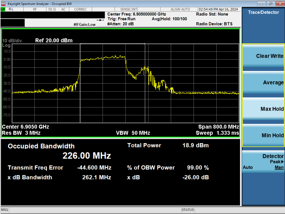
Plot 7-80. Occupied Bandwidth Plot MIMO ANT2 (320MHz BW 802. 11be (Full Tones) (UNII Band 8) – Ch. 191)
