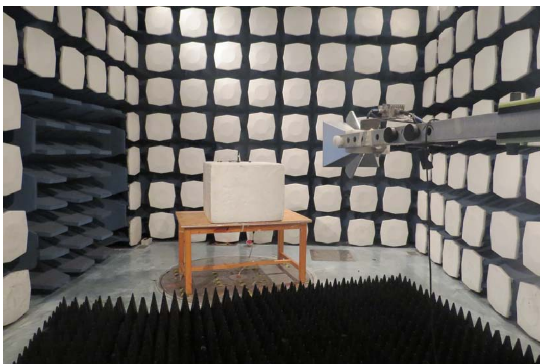
Picture 2: Radiated Spurious Emissions Test setup
