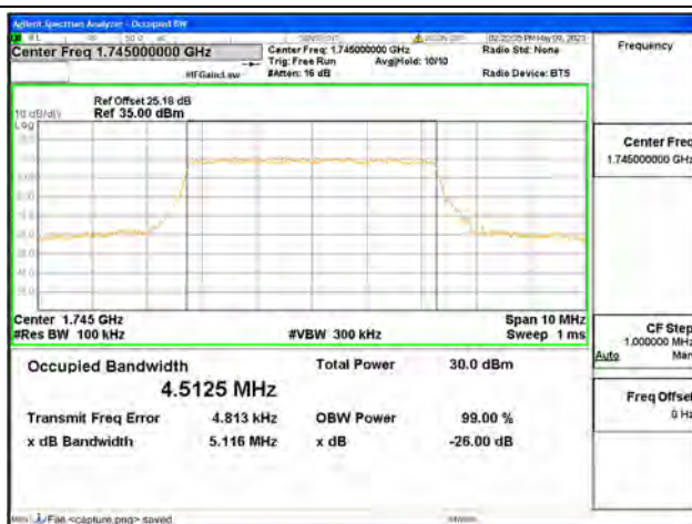
Band66 / 5MHz / 16QAM/ Mid CH
