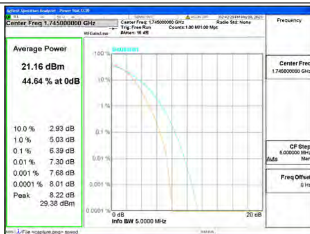
Band66 / 5MHz / Mid CH / 16QAM
