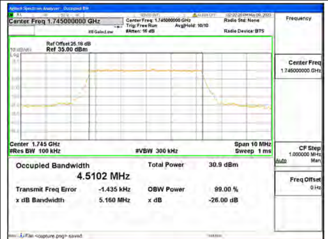
Band66 / 5MHz / QPSK/ Mid CH
