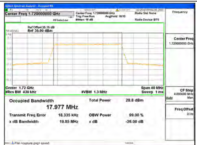
Band66 / 20MHz / 64QAM/ Low CH
