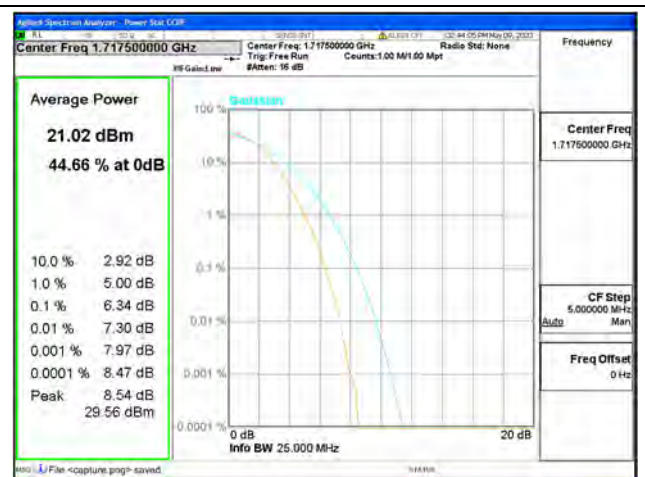
Band66 / 15MHz / Low CH / 16QAM
