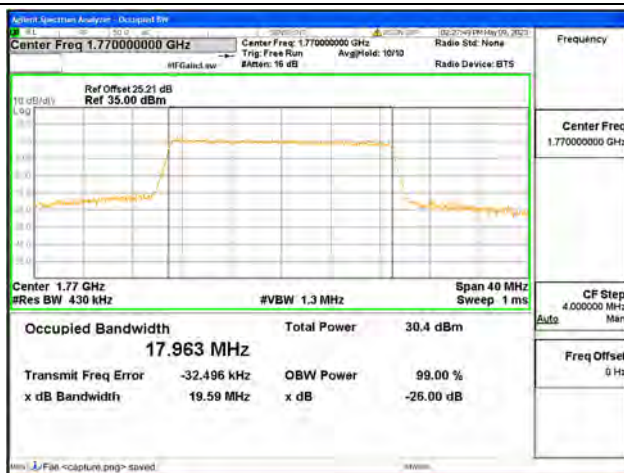
Band66 / 20MHz / 16QAM/ High CH
