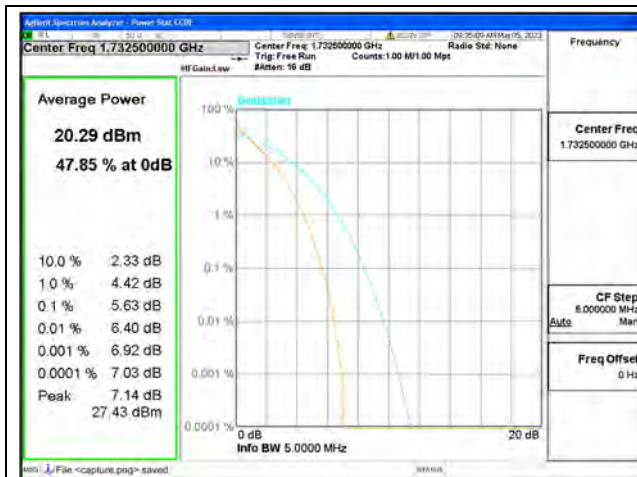
Band4 / 3MHz / Mid CH / QPSK
