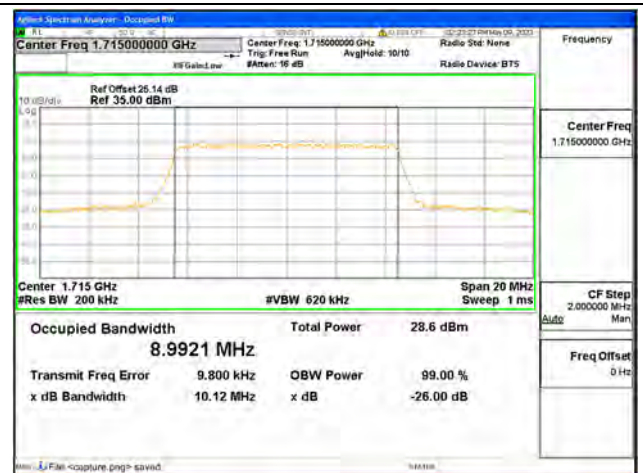
Band66 / 10MHz / 64QAM/ Low CH
