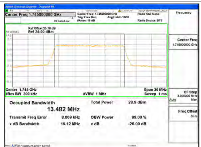
Band66 / 15MHz / 64QAM/ Mid CH
