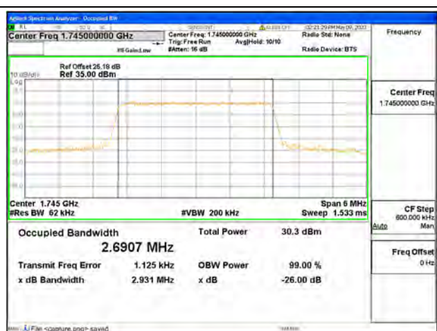
Band66 / 3MHz / 16QAM/ Mid CH
