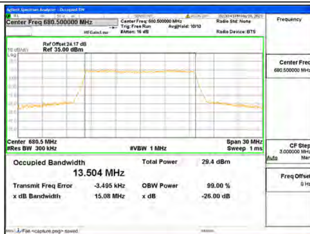
Band71 / 15MHz / 16QAM/ Mid CH
