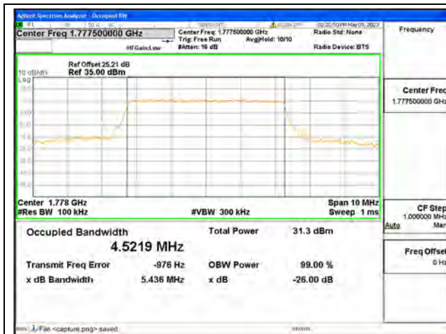
Band66 / 5MHz / QPSK/ High CH
