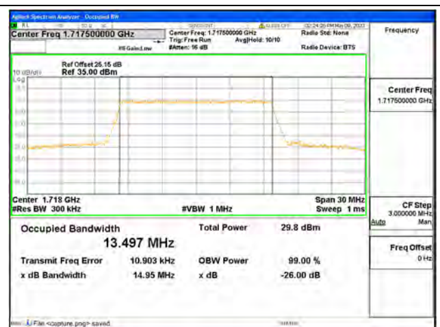
Band66 / 15MHz / 16QAM/ Low CH
