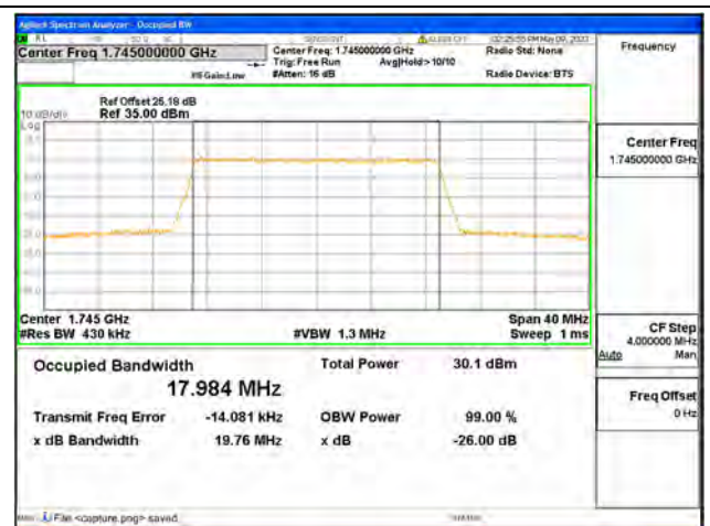
Band66 / 20MHz / 16QAM/ Mid CH
