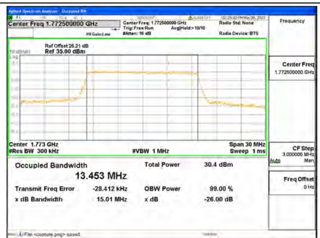
Band66 / 15MHz / 16QAM/ High CH
