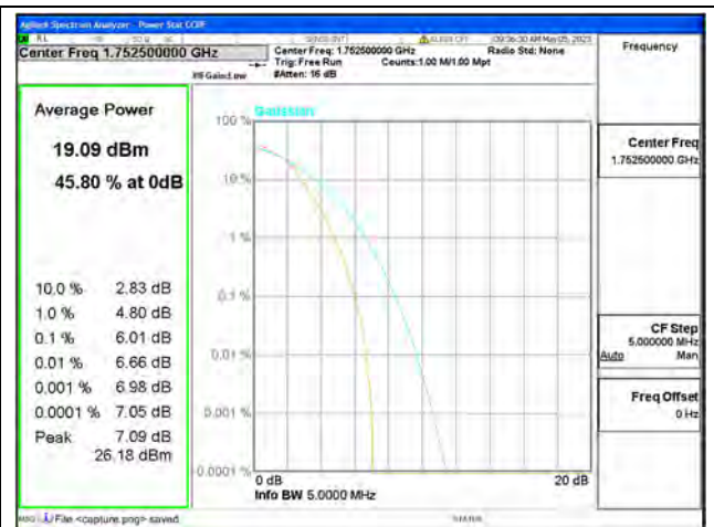
Band4 / 5MHz / High CH / 16QAM
