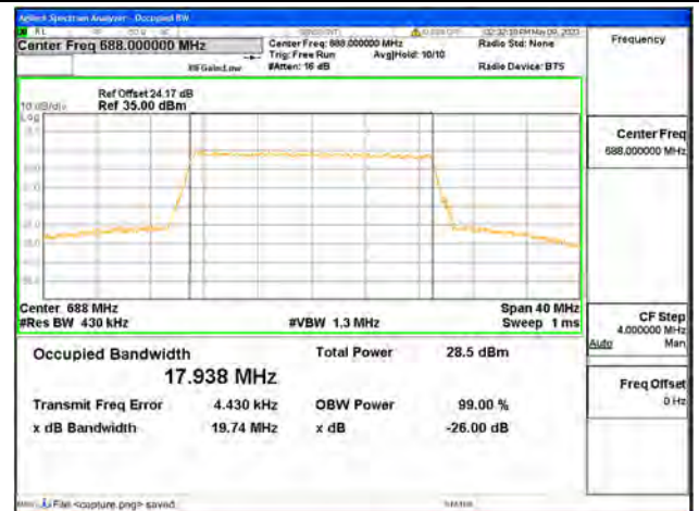
Band71 / 20MHz / 64QAM/ High CH
