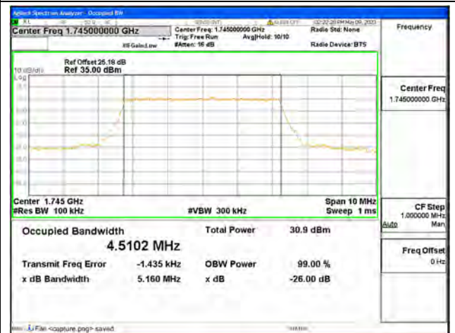
Band66 / 5MHz / QPSK/ Mid CH
