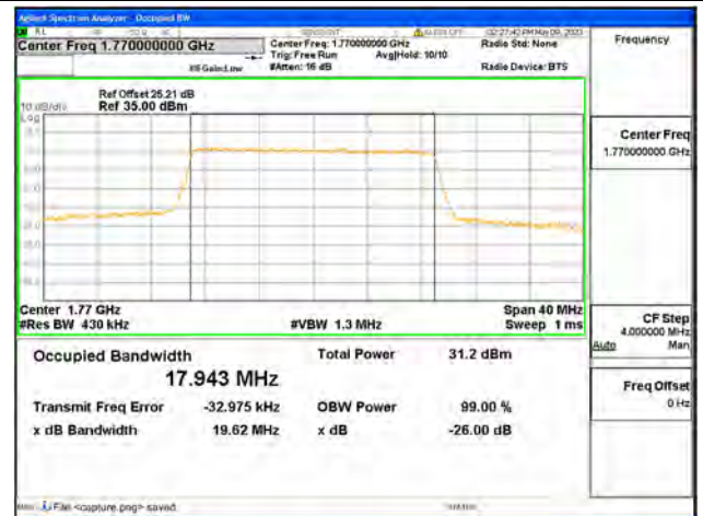
Band66 / 20MHz / QPSK/ High CH
