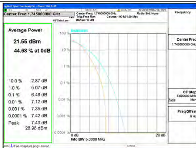
Band66 / 1.4MHz / Mid CH / 16QAM
