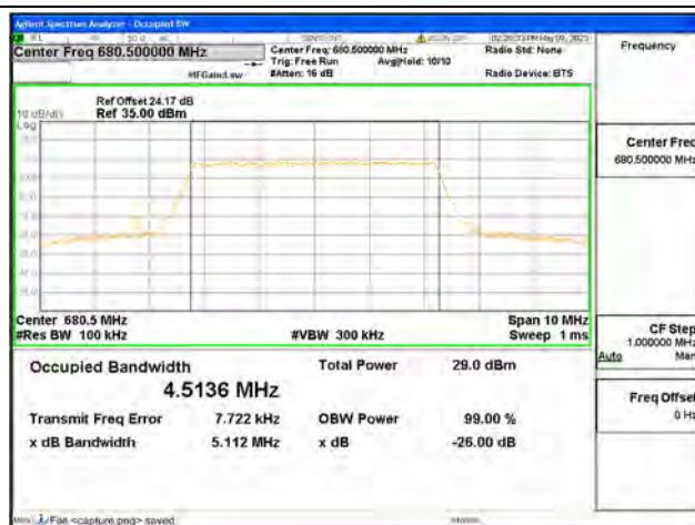
Band71 / 5MHz / 16QAM/ Mid CH
