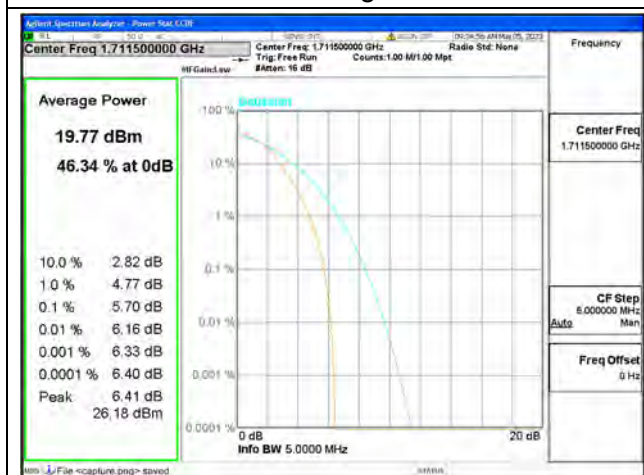
Band4 / 3MHz / Low CH / 16QAM
