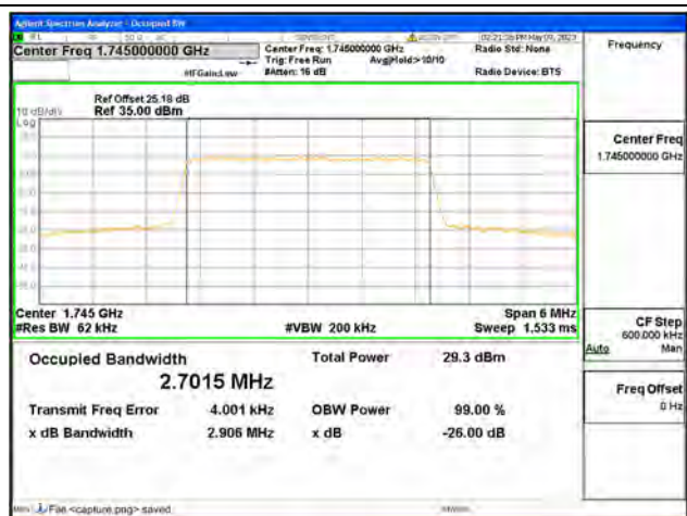
Band66 / 3MHz / 64QAM/ Mid CH
