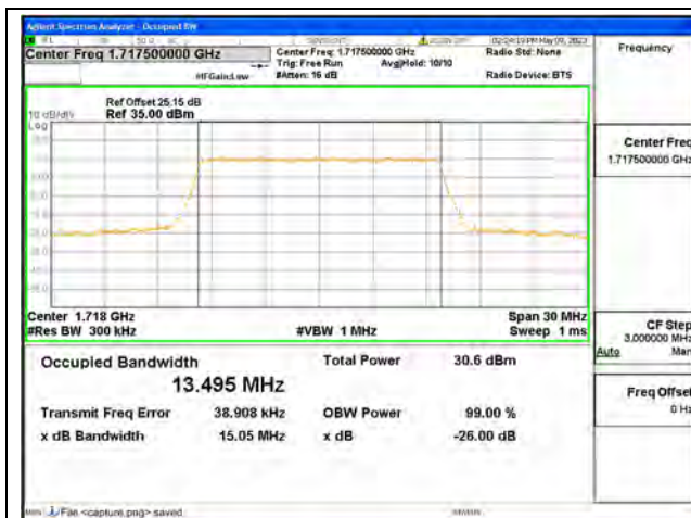
Band66 / 15MHz / QPSK/ Low CH
