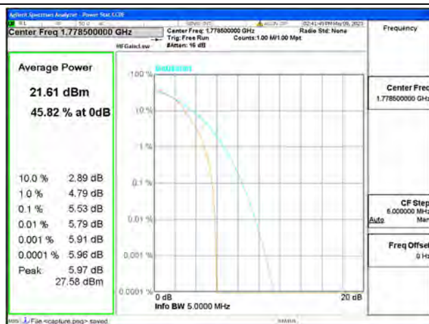
Band66 / 3MHz / High CH / 16QAM
