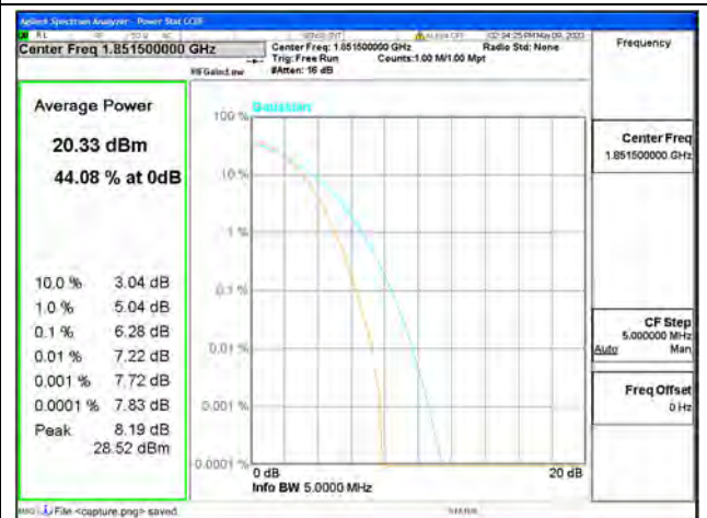
Band25 / 3MHz / Low CH / 64QAM
