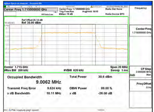
Band66 / 10MHz / QPSK/ Low CH
