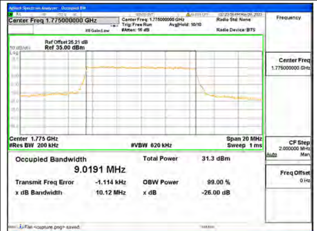
Band66 / 10MHz / QPSK/ High CH
