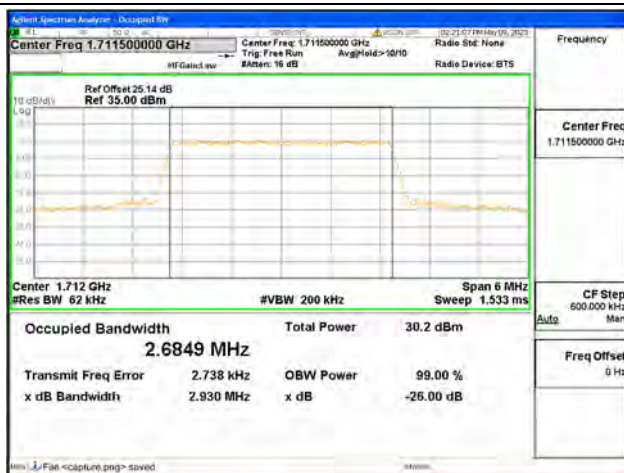
Band66 / 3MHz / 16QAM/ Low CH
