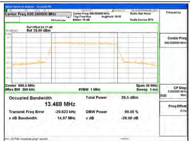
Band71 / 15MHz / 16QAM/ High CH
