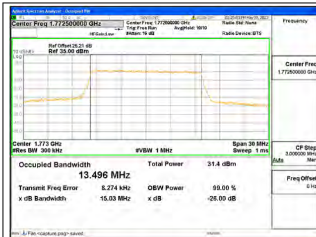
Band66 / 15MHz / QPSK/ High CH
