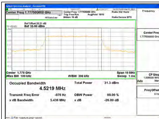
Band66 / 5MHz / QPSK/ High CH
