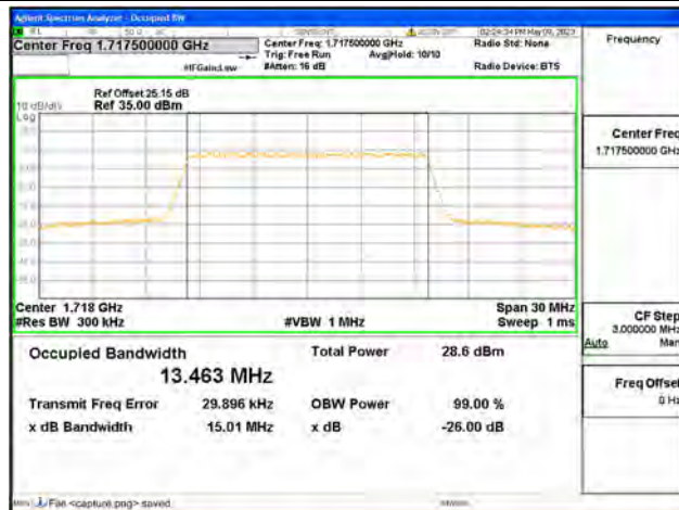
Band66 / 15MHz / 64QAM/ Low CH
