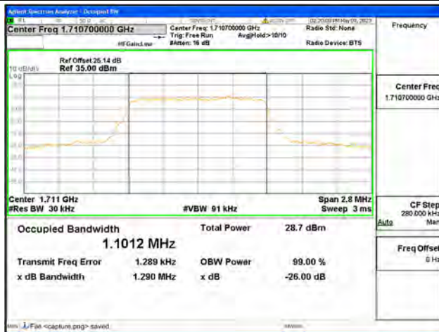
Band66 / 1.4MHz / 64QAM/ Low CH
