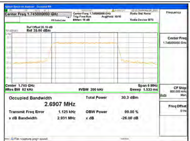
Band66 / 3MHz / 16QAM/ Mid CH
