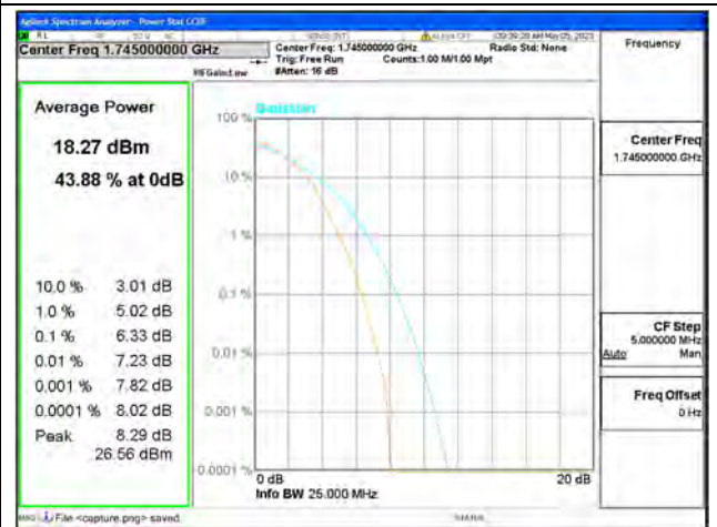
Band4 / 20MHz / High CH / 64QAM
