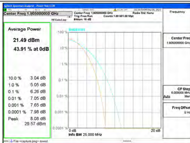
Band25 / 20MHz / High CH / 16QAM
