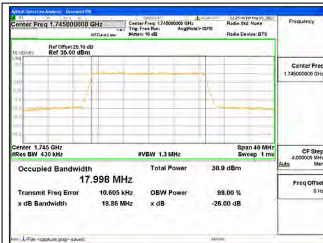
Band66 / 20MHz / QPSK/ Mid CH
