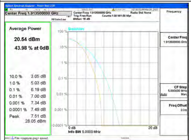
Band25 / 3MHz / High CH / 64QAM
