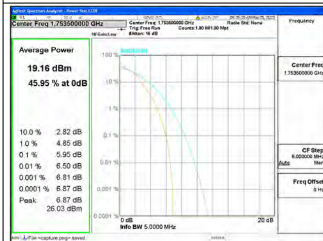
Band4 / 3MHz / High CH / 16QAM
