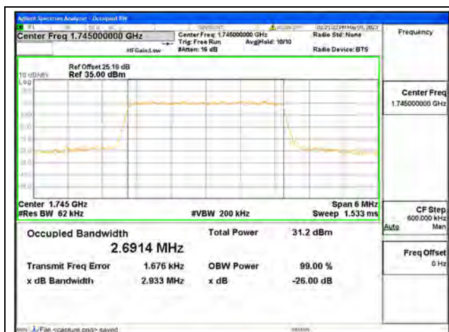
Band66 / 3MHz / QPSK/ Mid CH
