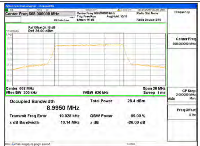
Band71 / 10MHz / 64QAM/ Low CH
