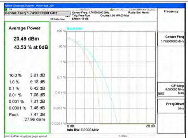
Band66 / 1.4MHz / Mid CH / 64QAM
