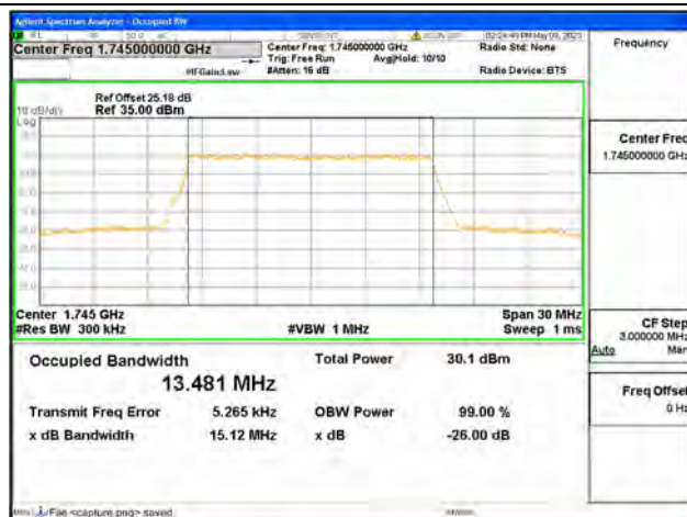
Band66 / 15MHz / 16QAM/ Mid CH
