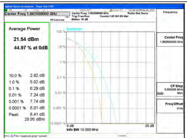
Band25 / 10MHz / Mid CH / 16QAM
