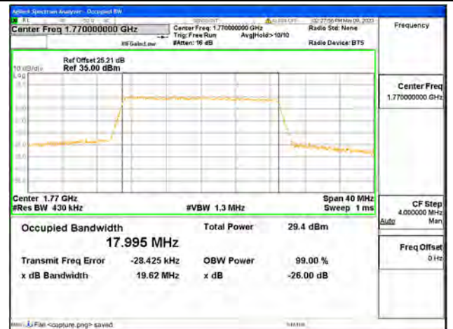
Band66 / 20MHz / 64QAM/ High CH
