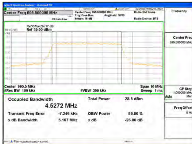
Band71 / 5MHz / 64QAM/ High CH
