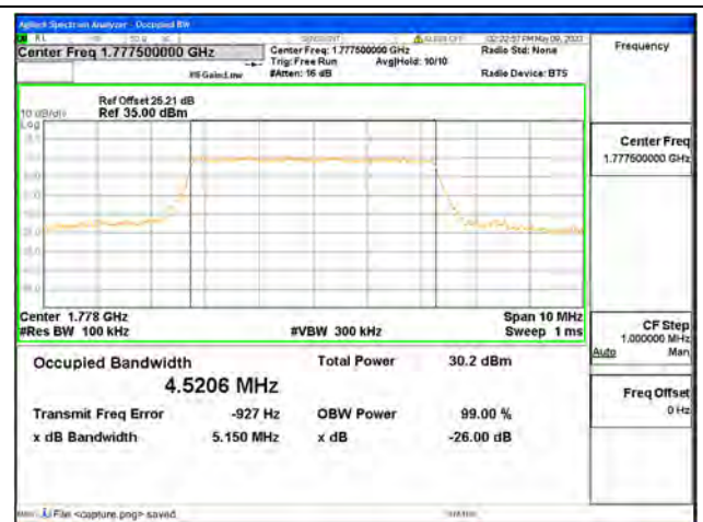
Band66 / 5MHz / 16QAM/ High CH
