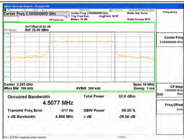
Band41 / 5MHz / 64QAM/ Mid CH
