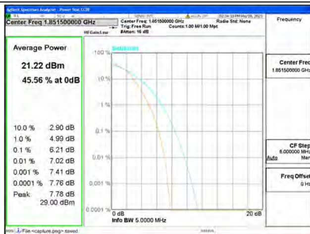
Band25 / 3MHz / Low CH / 16QAM
