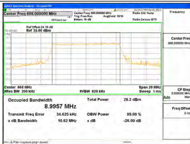
Band71 / 10MHz / 16QAM/ Low CH
