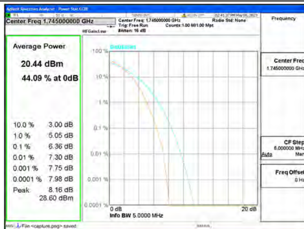
Band66 / 3MHz / Mid CH / 64QAM
