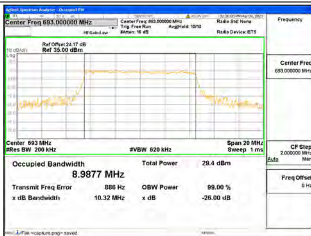
Band71 / 10MHz / 16QAM/ High CH
