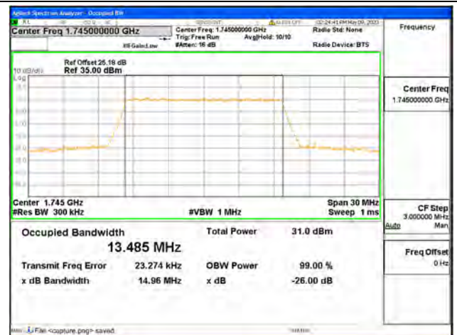
Band66 / 15MHz / QPSK/ Mid CH
