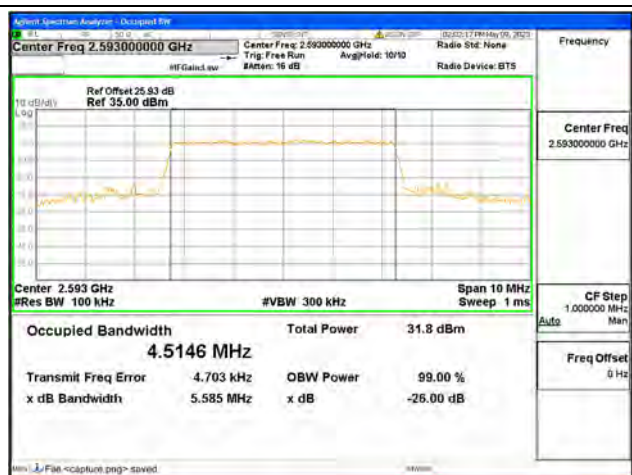
Band41 / 5MHz / 16QAM/ Mid CH
