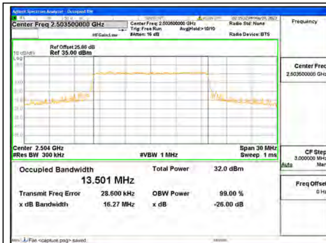
Band41 / 15MHz / QPSK/ Low CH
