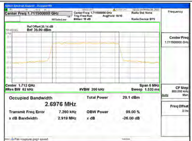
Band66 / 3MHz / 64QAM/ Low CH
