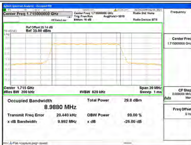
Band66 / 10MHz / 16QAM/ Low CH
