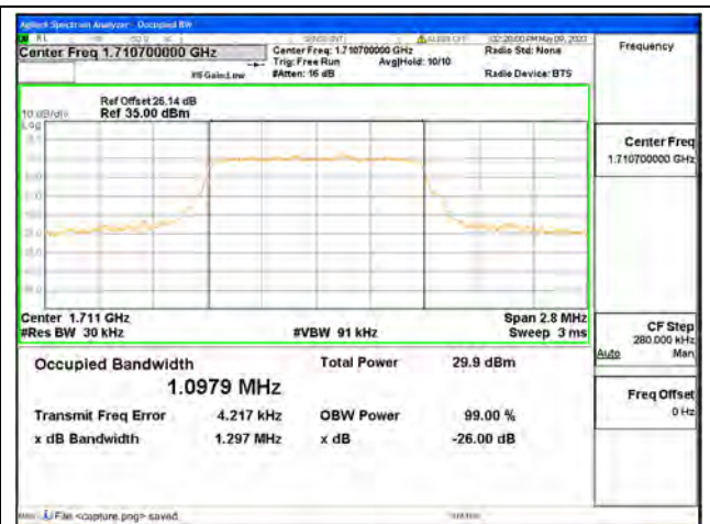
Band66 / 1.4MHz / 16QAM/ Low CH
