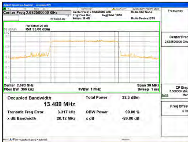
Band41 / 15MHz / 64QAM/ High CH
