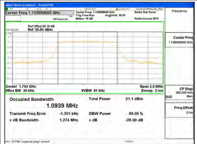
Band66 / 1.4MHz / QPSK/ Mid CH
