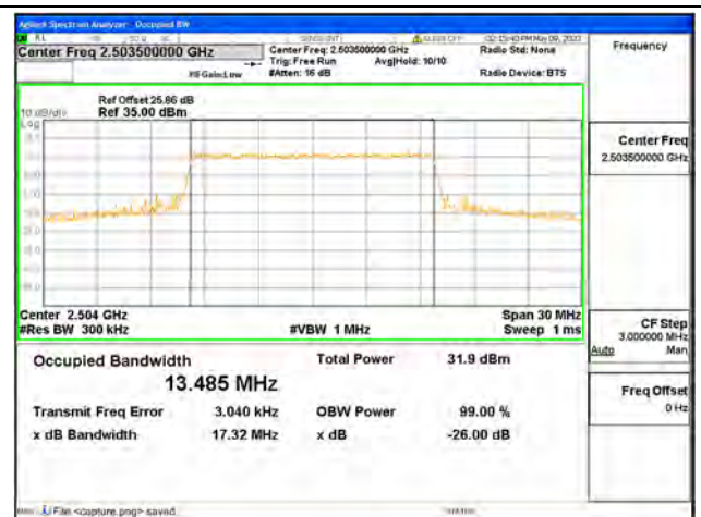
Band41 / 15MHz / 16QAM/ Low CH
