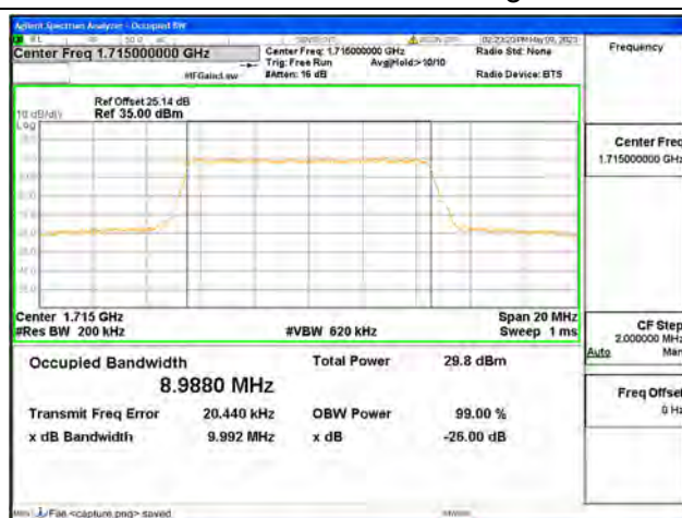
Band66 / 10MHz / 16QAM/ Low CH
