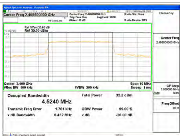
Band41 / 5MHz / 16QAM/ Low CH
