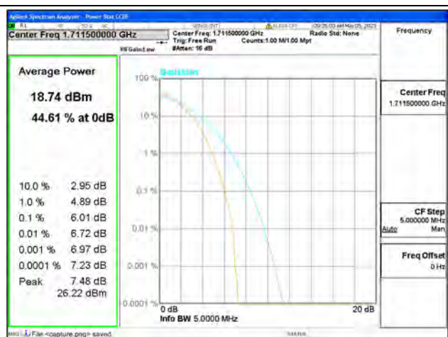
Band4 / 3MHz / Low CH / 64QAM
