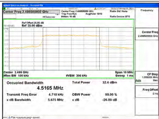
Band41 / 5MHz / 64QAM/ Low CH
