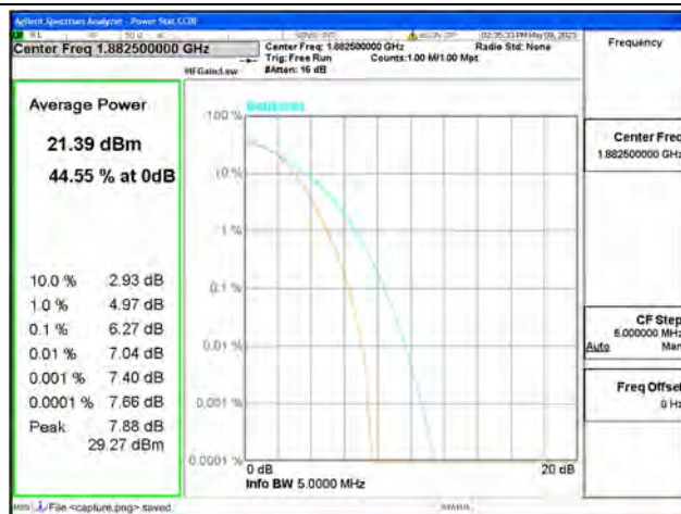
Band25 / 5MHz / Mid CH / 16QAM
