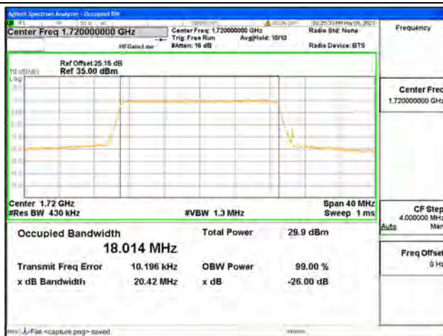
Band66 / 20MHz / 16QAM/ Low CH
