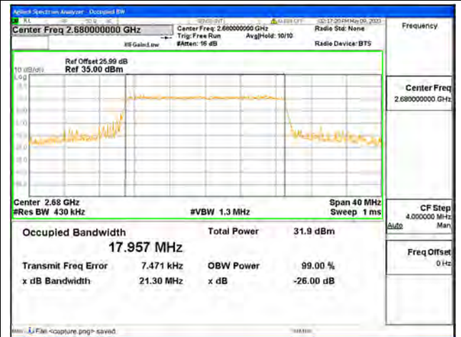
Band41 / 20MHz / QPSK/ High CH
