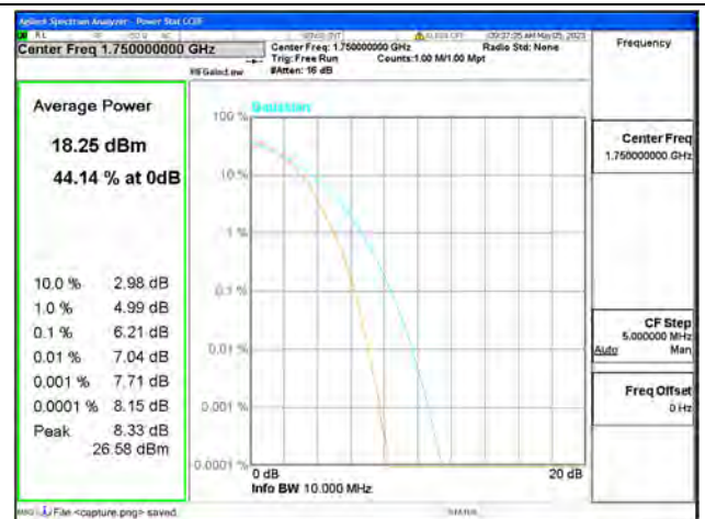
Band4 / 10MHz / High CH / 64QAM
