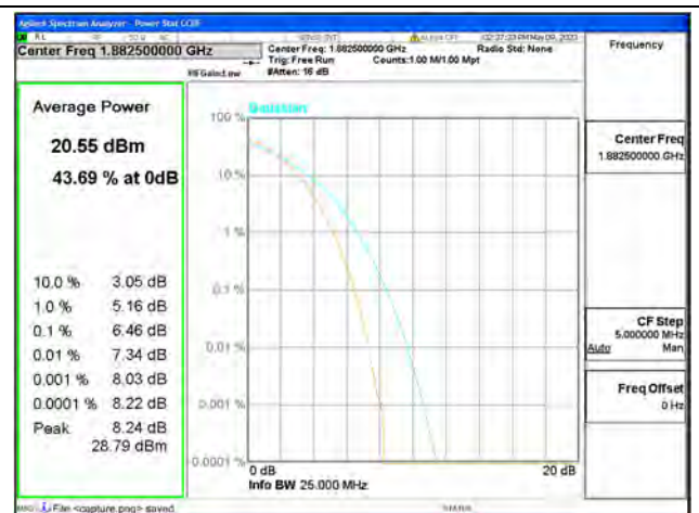
Band25 / 15MHz / Mid CH / 64QAM
