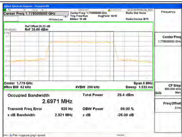
Band66 / 3MHz / 64QAM/ High CH
