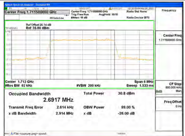
Band66 / 3MHz / QPSK/ Low CH
