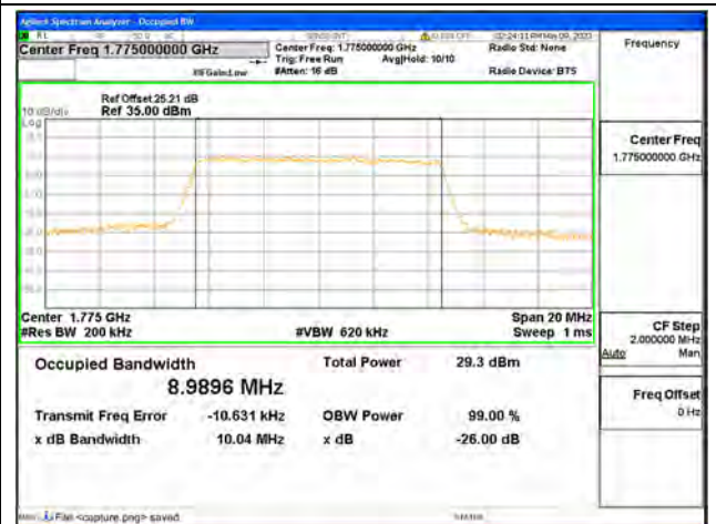
Band66 / 10MHz / 64QAM/ High CH
