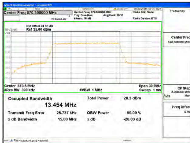
Band71 / 15MHz / 64QAM/ Low CH
