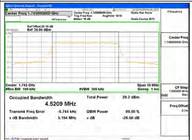
Band66 / 5MHz / 64QAM/ Mid CH
