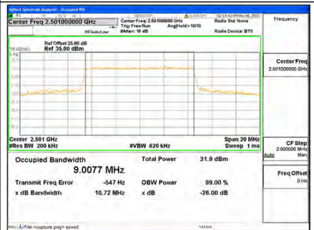
Band41 / 10MHz / 64QAM/ Low CH
