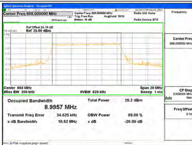
Band71 / 10MHz / 16QAM/ Low CH
