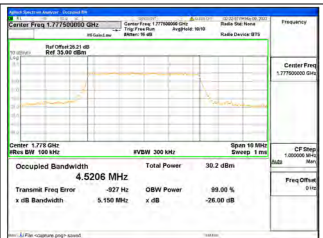
Band66 / 5MHz / 16QAM/ High CH
