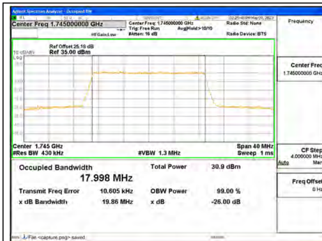
Band66 / 20MHz / QPSK/ Mid CH
