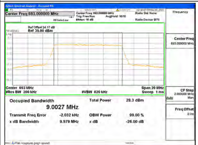
Band71 / 10MHz / 64QAM/ High CH
