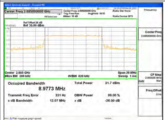
Band41 / 10MHz / 64QAM/ High CH
