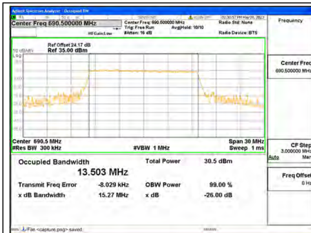
Band71 / 15MHz / QPSK/ High CH
