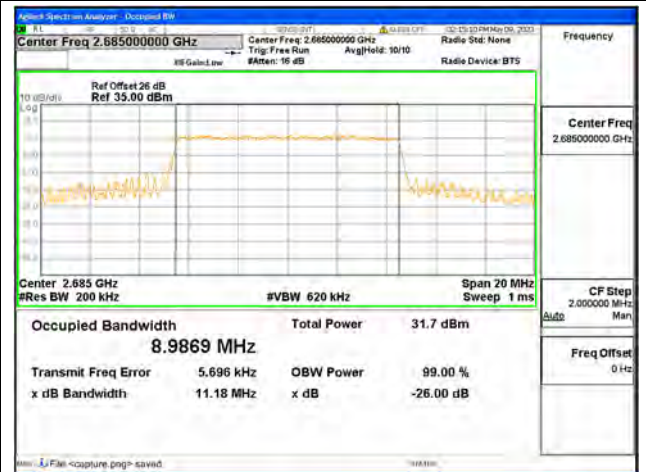
Band41 / 10MHz / QPSK/ High CH
