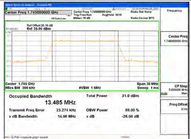
Band66 / 15MHz / QPSK/ Mid CH
