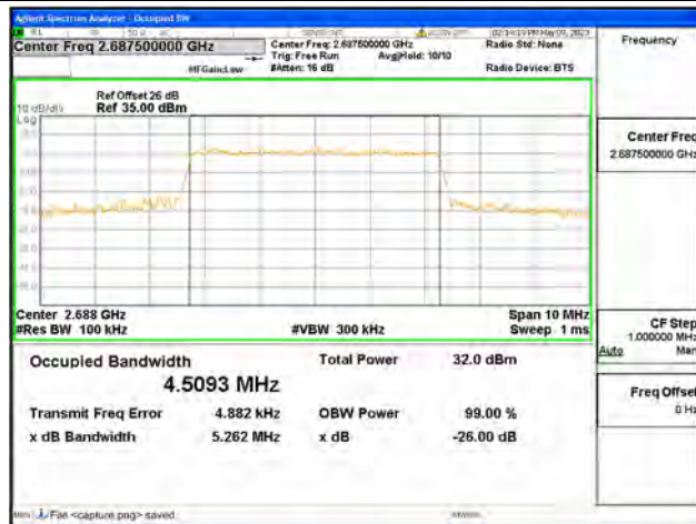
Band41 / 5MHz / 64QAM/ High CH
