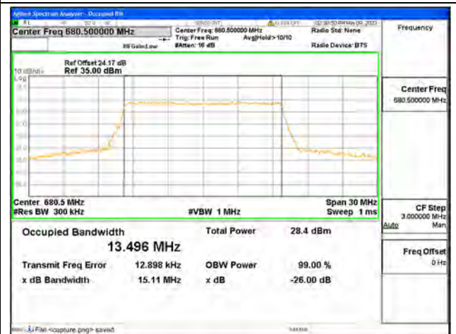
Band71 / 15MHz / 64QAM/ Mid CH
