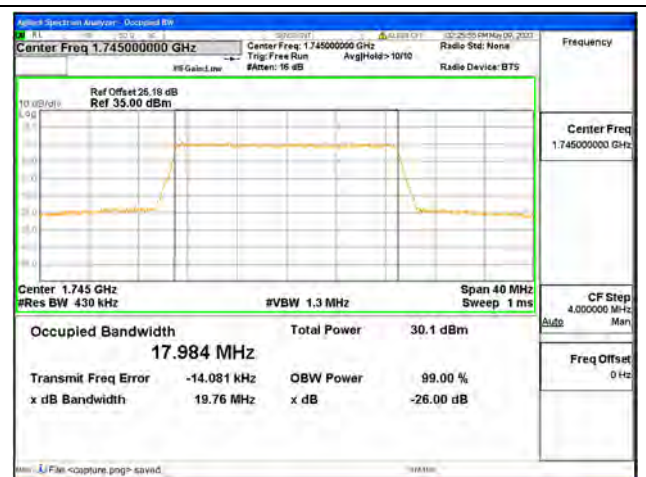
Band66 / 20MHz / 16QAM/ Mid CH
