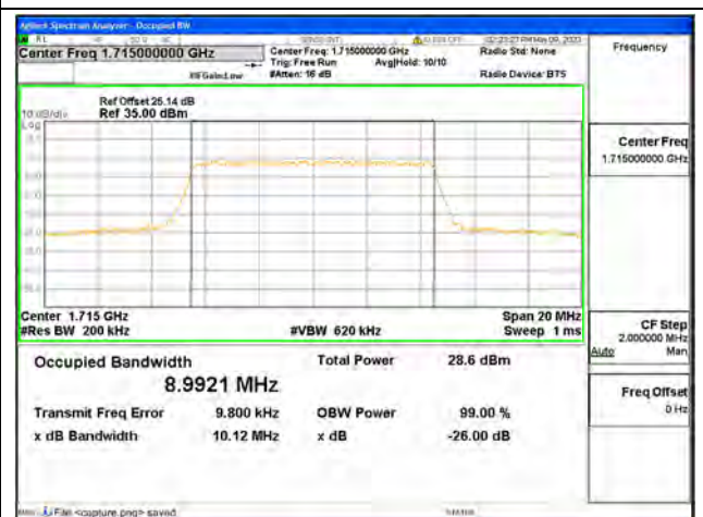
Band66 / 10MHz / 64QAM/ Low CH
