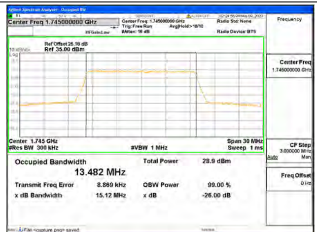
Band66 / 15MHz / 64QAM/ Mid CH
