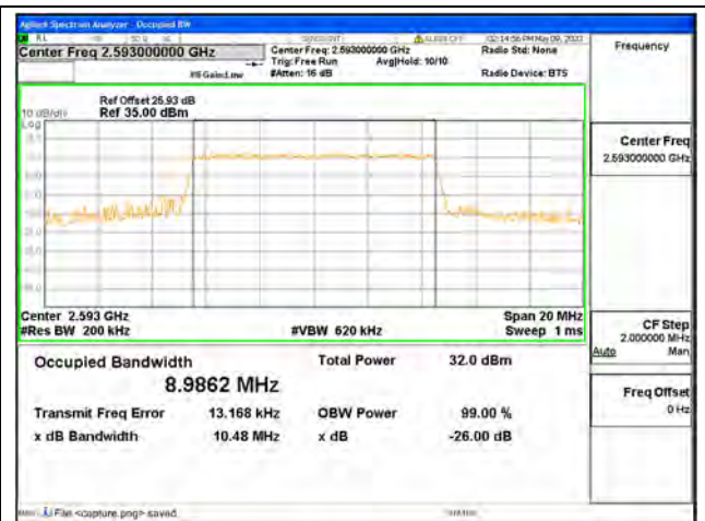
Band41 / 10MHz / 16QAM/ Mid CH
