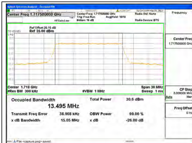
Band66 / 15MHz / QPSK/ Low CH
