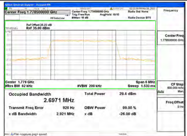
Band66 / 3MHz / 64QAM/ High CH
