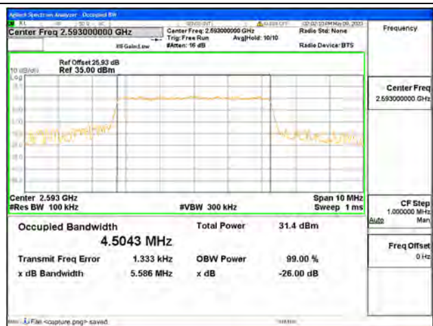
Band41 / 5MHz / QPSK/ Mid CH
