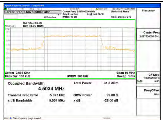
Band41 / 5MHz / 16QAM/ High CH
