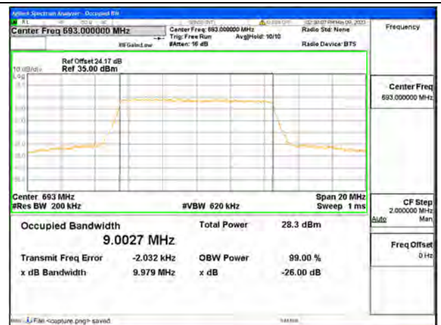
Band71 / 10MHz / 64QAM/ High CH
