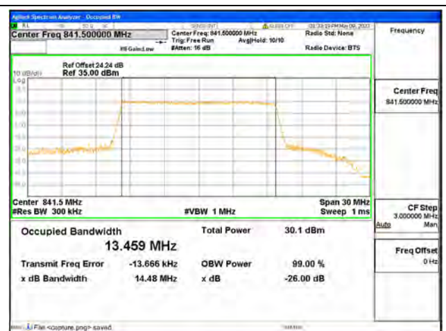
Band26 Part22 / 15MHz / 16QAM/ High CH
