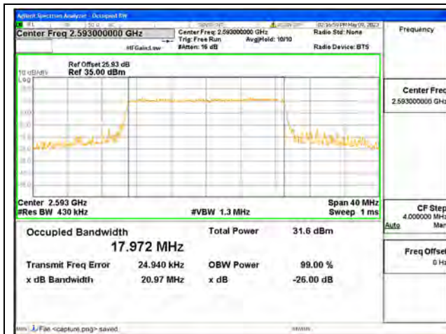
Band41 / 20MHz / QPSK/ Mid CH
