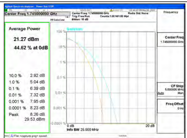
Band66 / 20MHz / Mid CH / 16QAM
