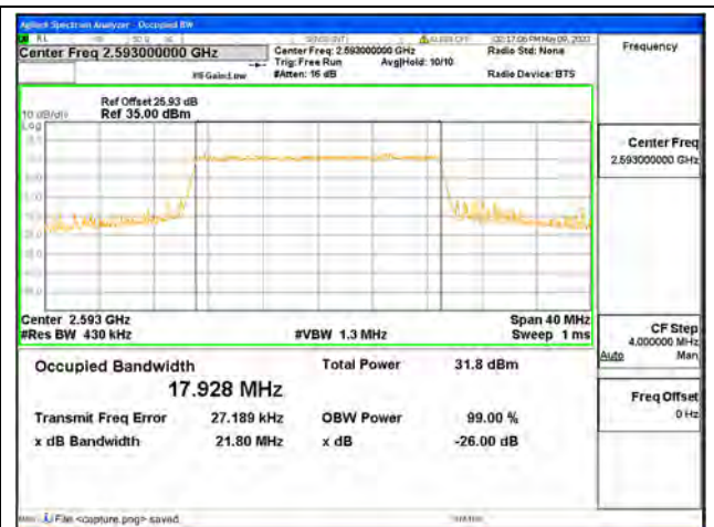
Band41 / 20MHz / 16QAM/ Mid CH
