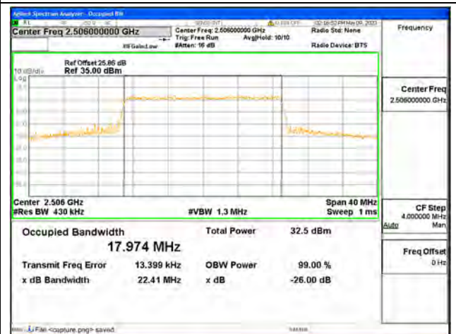
Band41 / 20MHz / 64QAM/ Low CH
