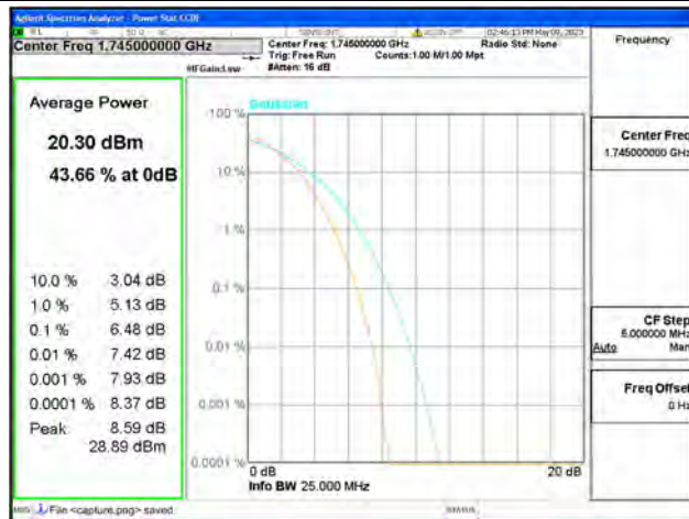
Band66 / 20MHz / Mid CH / 64QAM
