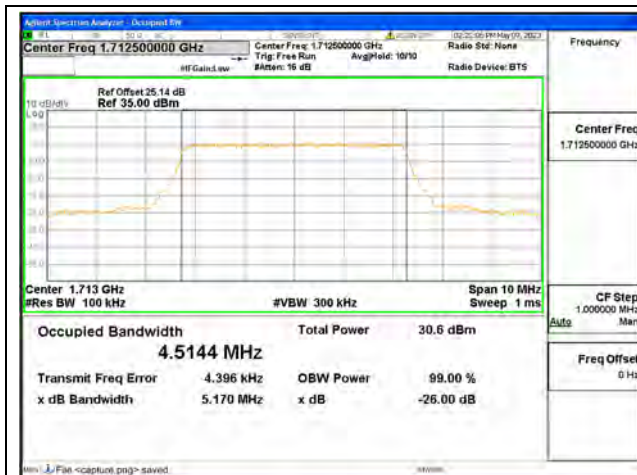
Band66 / 5MHz / QPSK/ Low CH
