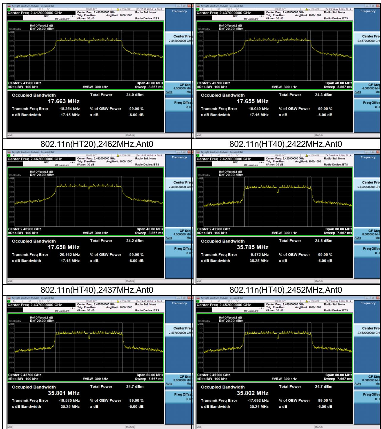
**TEST REPORT****3. Occupied Bandwidth****3.1 Test Data**
