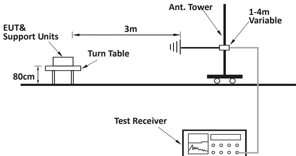
**TEST REPORT****For Radiated emission above 1GHz:**
