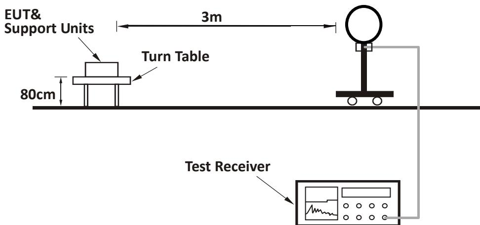
For Radiated emission 30MHz to 1GHz:
