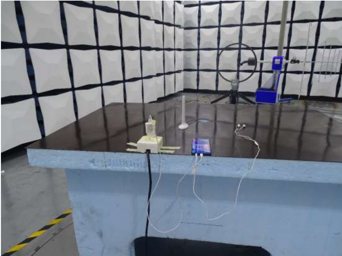
Radiated Spurious Emission (9K-30MHz)
