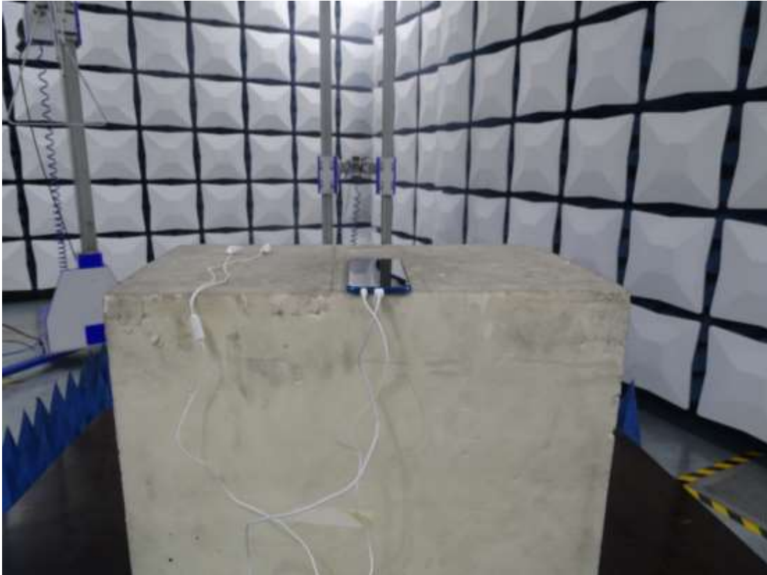
Radiated Spurious Emission (above 18GHz)
