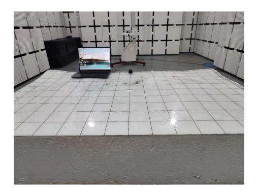
Set-up for Radiated Spurious Emission, Above 1GHz
