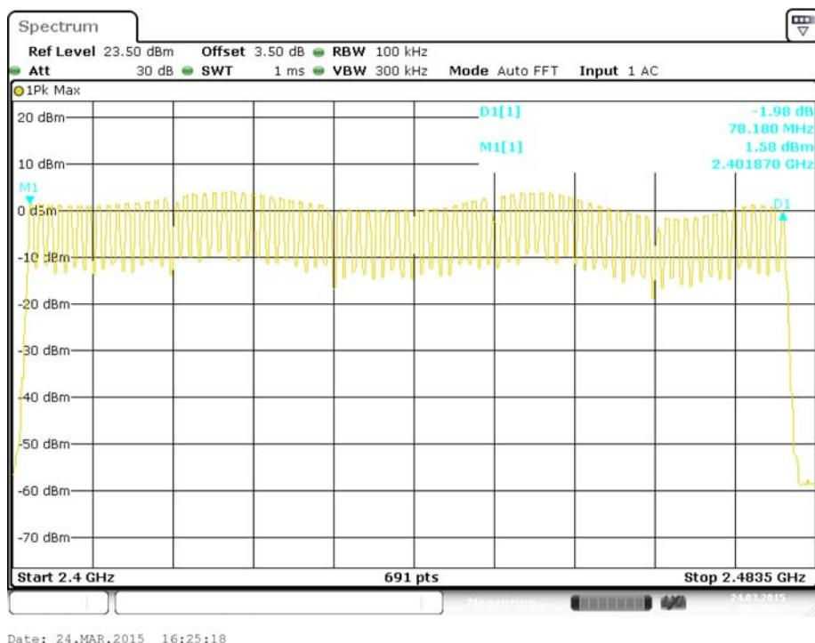
**EDR ( $\pi/4$ -DQPSK): Number of Hopping Channels**
