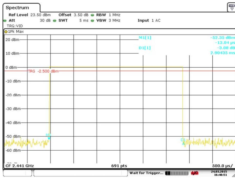
**Pulse time, High Channel, DH5**
