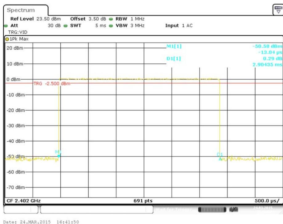
**Pulse time, Middle Channel, 2DH5**
