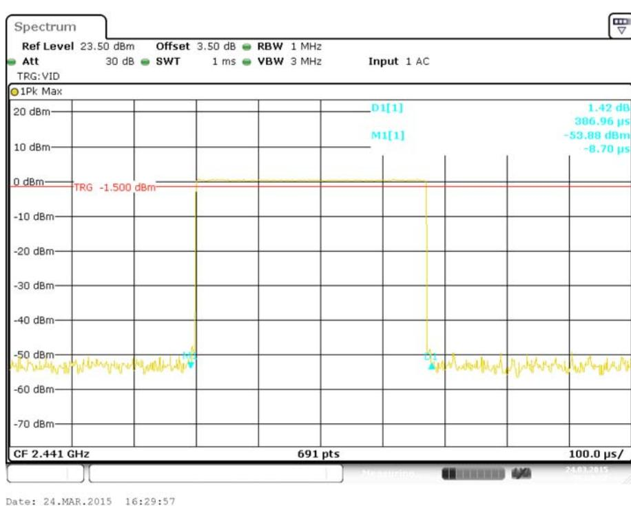
**Pulse time, High Channel, DH1**
