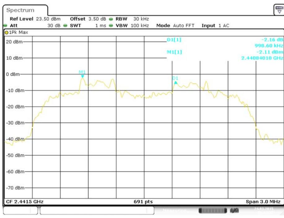
**EDR (8DPSK): High Channel**
