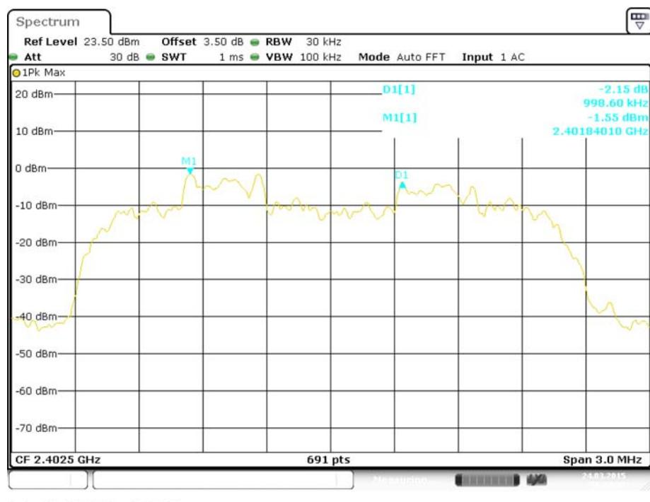
**EDR ( $\pi/4$ -DQPSK): Middle Channel**
