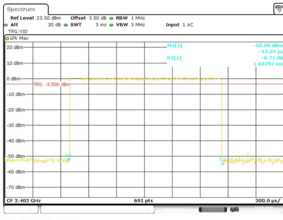
**Pulse time, Middle Channel, 3DH3**
