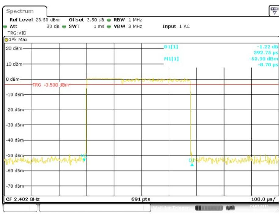
**Pulse time, Middle Channel, 2DH1**
