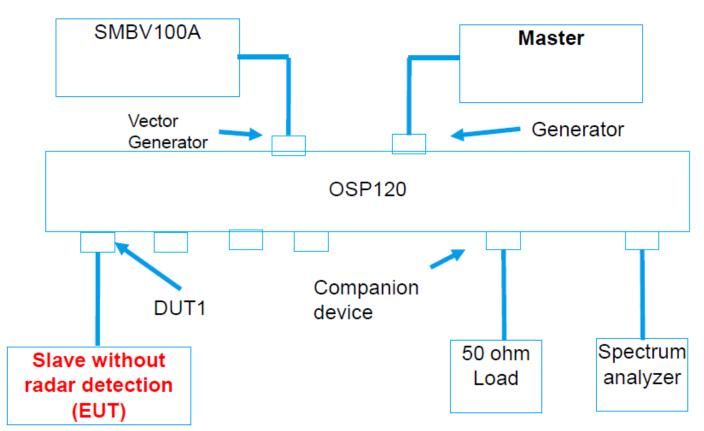
The UUT is a U-NII Device operating in Client mode without radar detection. The radar test signals are injected into the Master Device.
