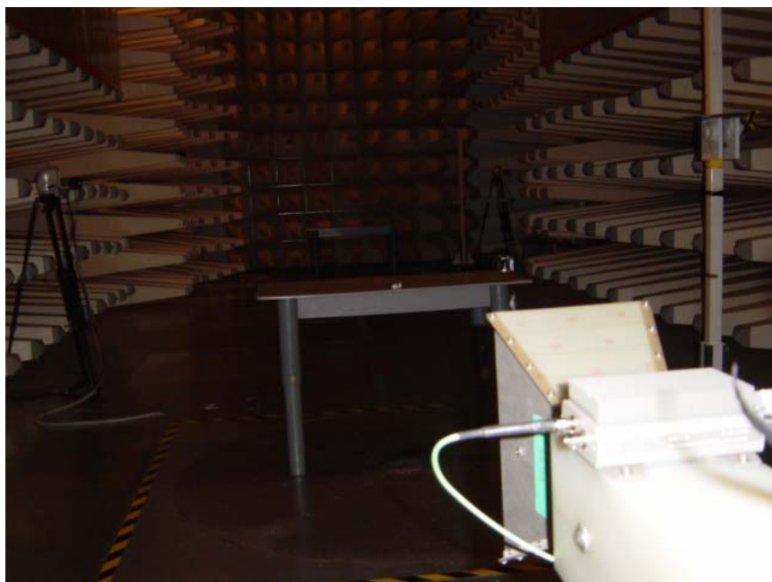
Set-up for Radiation Emission (reference photo)
