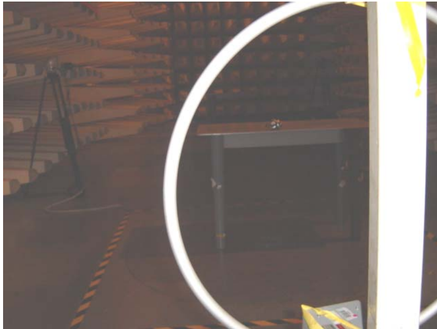
Set-up for Radiation Emission (Transceiver)
