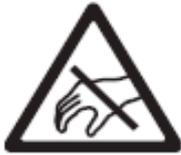
LED lamps used in the module are sensitive and can be damaged by ESD (electrostatic discharge). To prevent damage to LED lamps, do not touch when the device is running or switched off.
