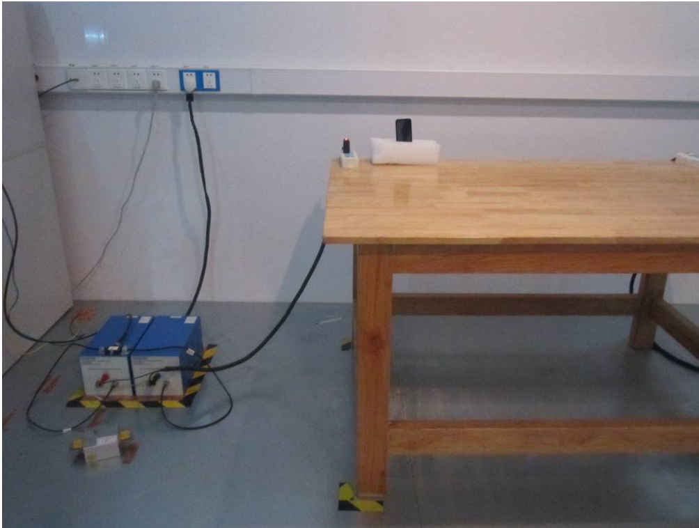
Conducted Emissions Test Setup Front View
