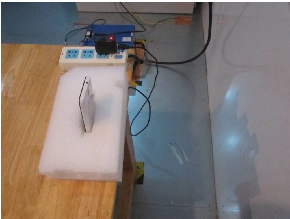
Conducted Emissions Test Setup Side View
