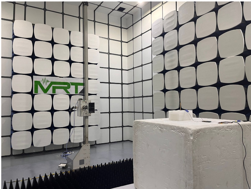
Description: Radiated Spurious Emission Test Setup for Ant 1 Above 1GHz
