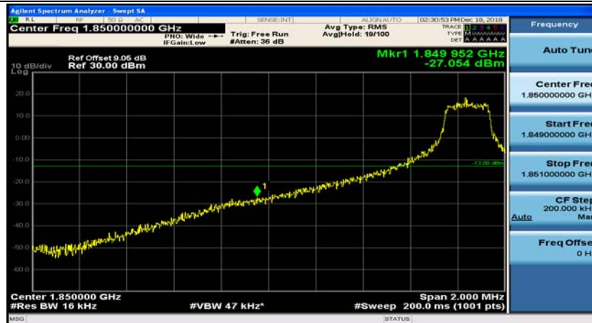
(Channel Bandwidth:15 MHz)_LCH_16QAM_1RB#37
