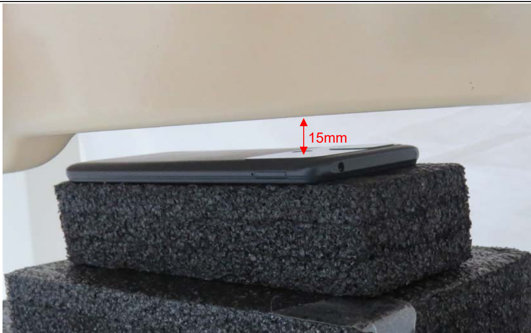
Picture 15: Back Side, the distance from handset to the bottom of the Phantom is 15mm
