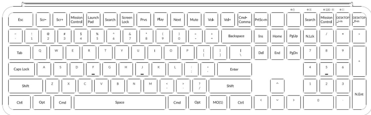
Layer 1: This layer will be activated when your keyboard's system toggle is switched to Mac and press the fn/MO(1) key.
