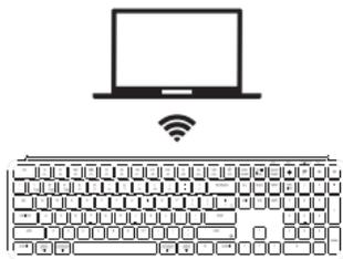
Connect the 2.4GHz receiver to the device USB port.
