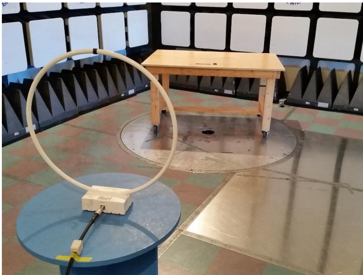
Figure 2 – Radiated Emissions Setup – Photo 1
