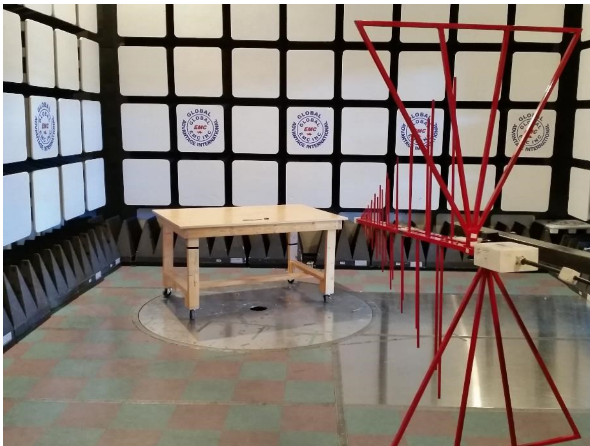
Figure 3 – Radiated Emissions Setup – Photo 2
