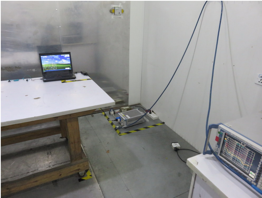
FCC RADIATED EMISSION TEST SETUP
