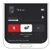
4 Go to More Settings > Sound Modes, select Low Gain Mode. In this mode, the maximum sound pressure level can reach 130 dB, effortlessly preventing sound spikes and distortion, while significantly improving recording quality.
