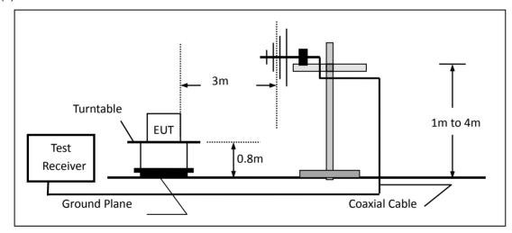
(c) For radiated emissions above 1000MHz
