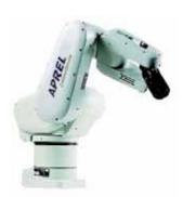
ALSAS-10U utilizes a six axis articulated robot, which is controlled using a Pentium based real-time movement controller. The movement kinematics engine utilizes proprietary (Thermo CRS) interpolation and extrapolation algorithms, which allow full freedom of movement for each of the six joints within the working envelope. Utilization of joint 6 allows for full probe rotation with a tolerance better than 0.05mm around the central axis.
