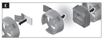
Use a commercially available two-part adhesive (not supplied) for attachment of the GCY 30-5 T to a power tool or industrial asset. Observe all processing instructions from the adhesive manufacturer. The use of other adhesives may be adequate depending on the application and environment. Choosing the right adhesive composition will create a long lasting bond between the GCY 30-5 T base and the tool.
