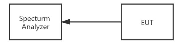
The EUT which is powered by the DC 5V, is connected to the Spectrum Analyzer; the RF load attached to the EUT antenna terminal is 50 Ohm; the path loss as the factor is calibrated to correct the reading. Make the measurement with the spectrum analyzer's resolution bandwidth(RBW) = 100 kHz. In order to make an accurate measurement, set the span greater than RBW.
