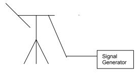
The spectrum analyzer is monitored to verify that the output of the signal generator produces a signal equal in amplitude to a previously measured spurious emission.
