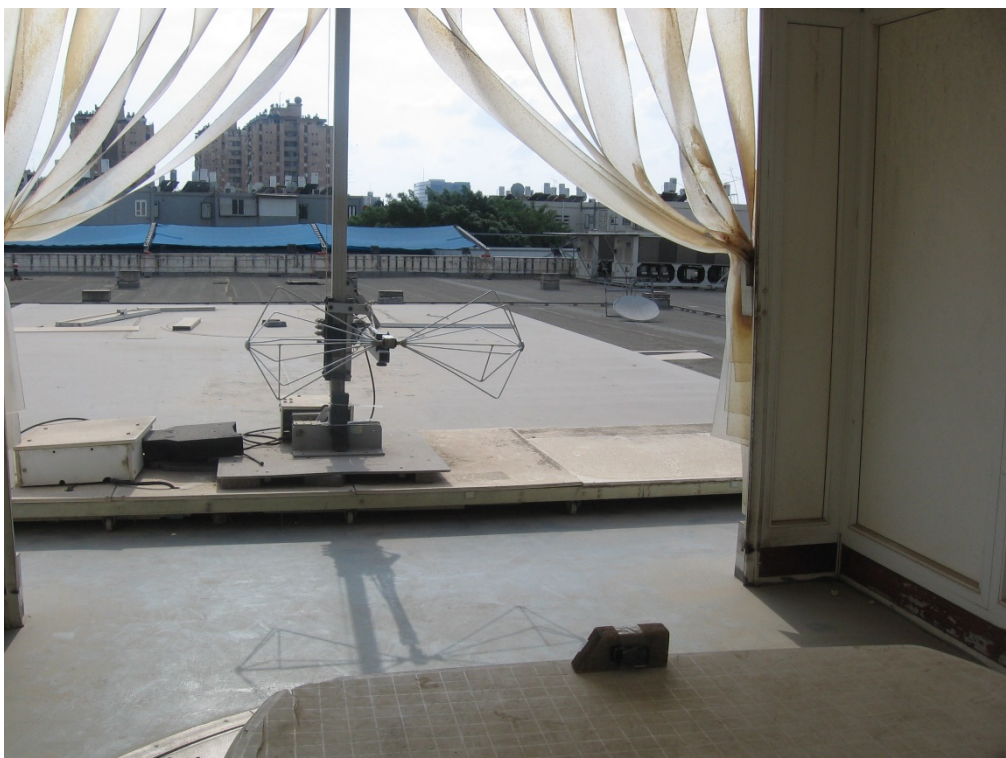
Radiated Emission Test, 30-200MHz
