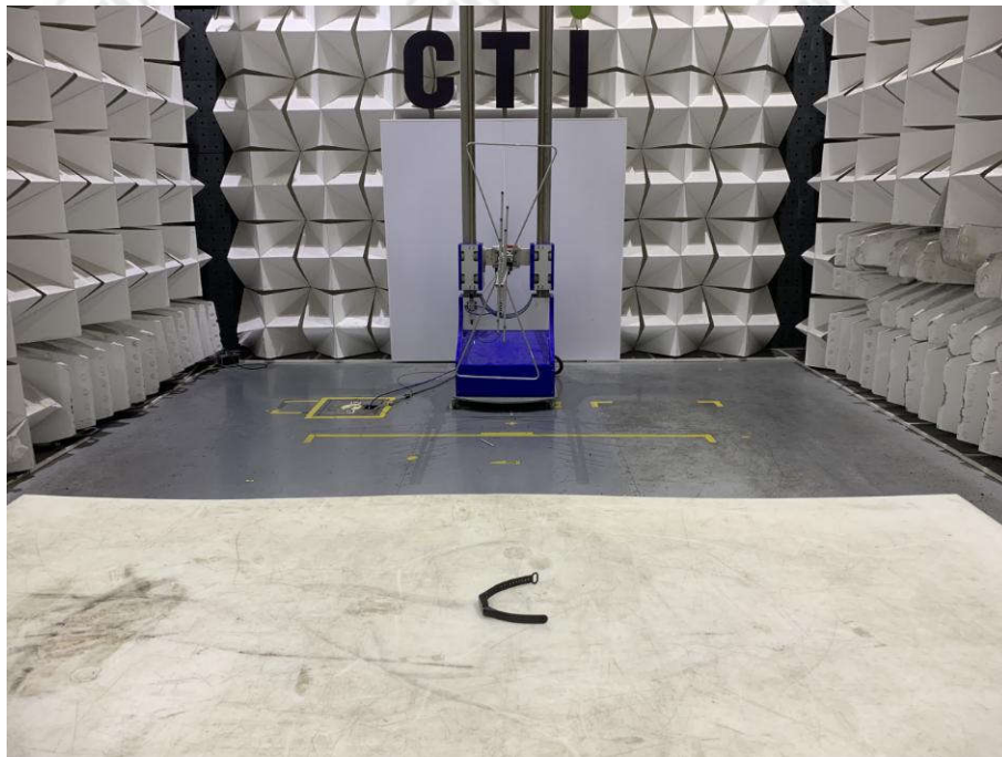
Radiated spurious emission Test Setup-1(Below 1GHz)
