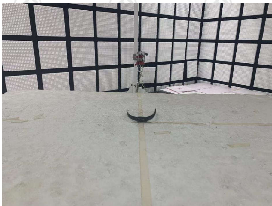
Radiated spurious emission Test Setup-2(Above 1GHz)
