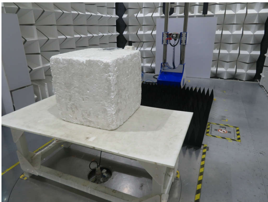
Radiated spurious emission Test Setup-3(Above 1GHz)
