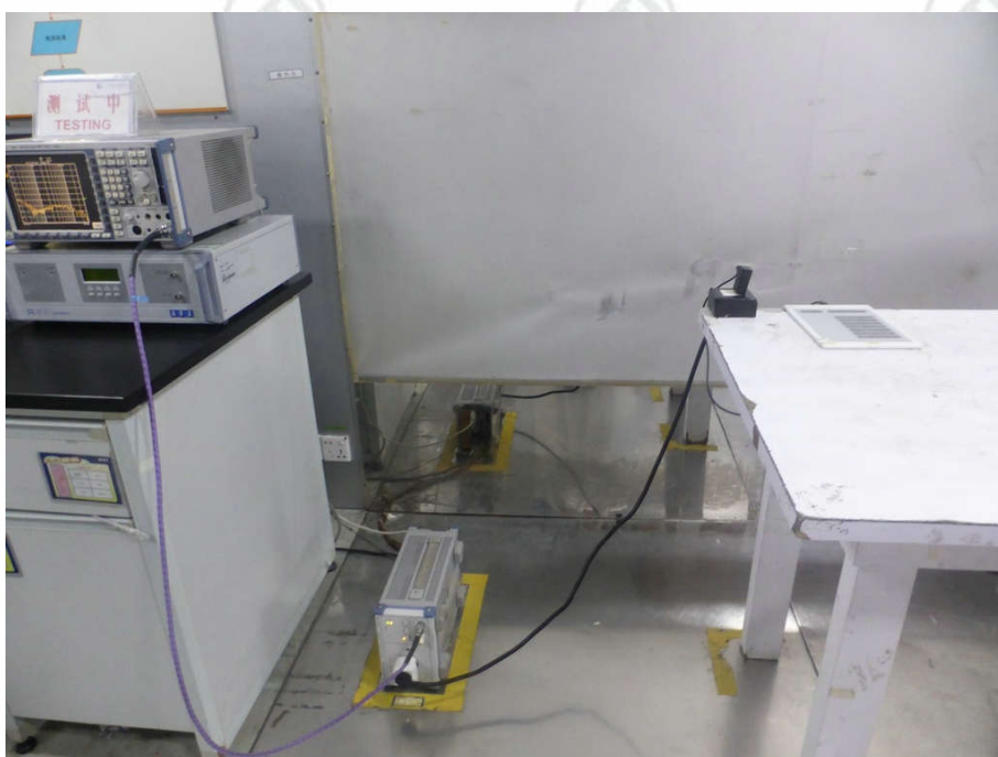
Conducted Emissions Test Setup
