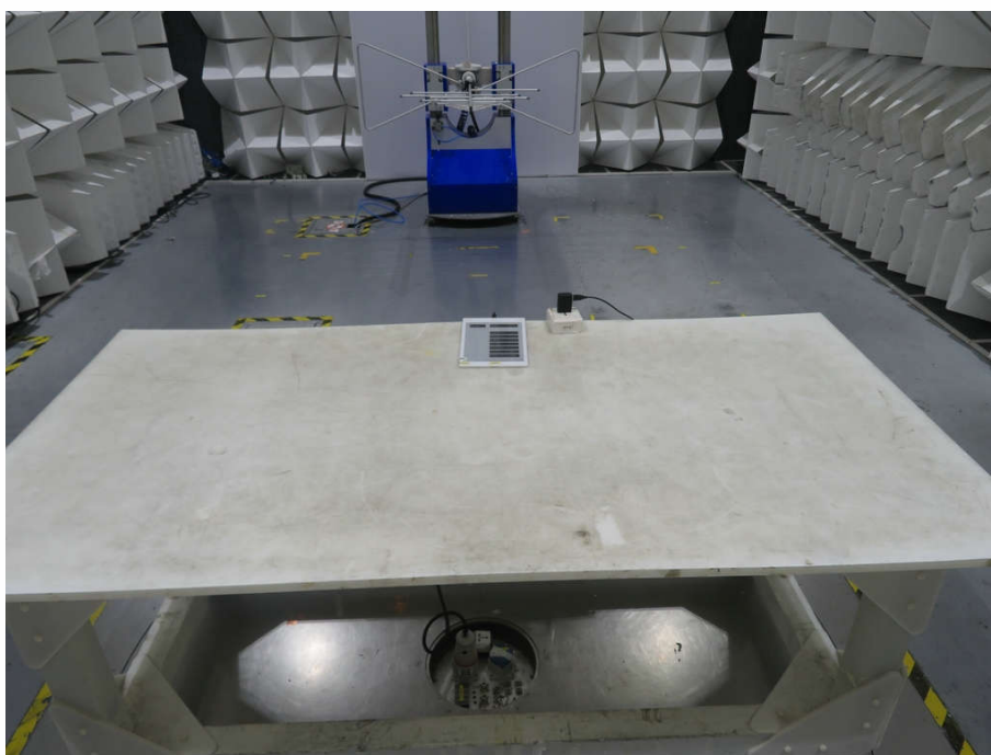
Radiated spurious emission Test Setup-2(30MHz-1GHz)
