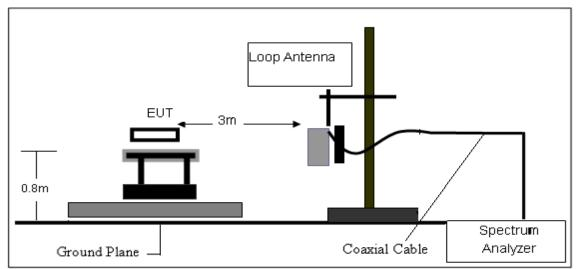
2. Radiated Emission Test-Up Frequency 30MHz~1GHz
