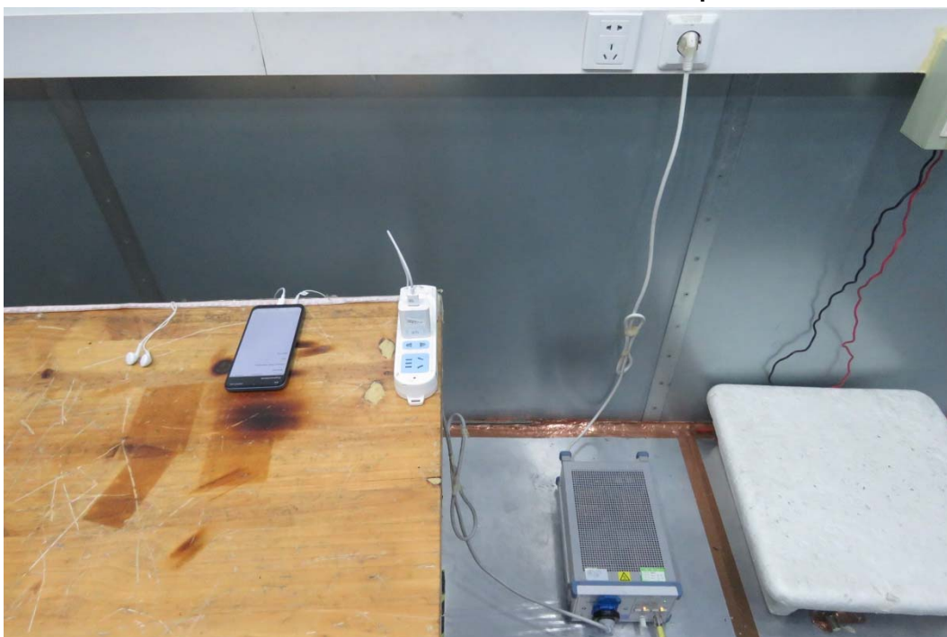
Picture 2 Conducted Emission Test Setup
