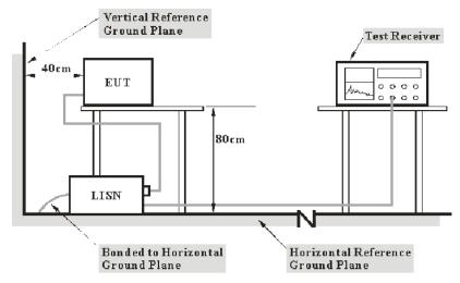
Note: 1. Support units were connected to second LISN.2. Both of LISNs (AMN) 80 cm from EUT and at the least 80 cm from other units and other metal planes support units.
