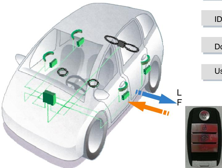
**Figure 1: Principle of Communication**
