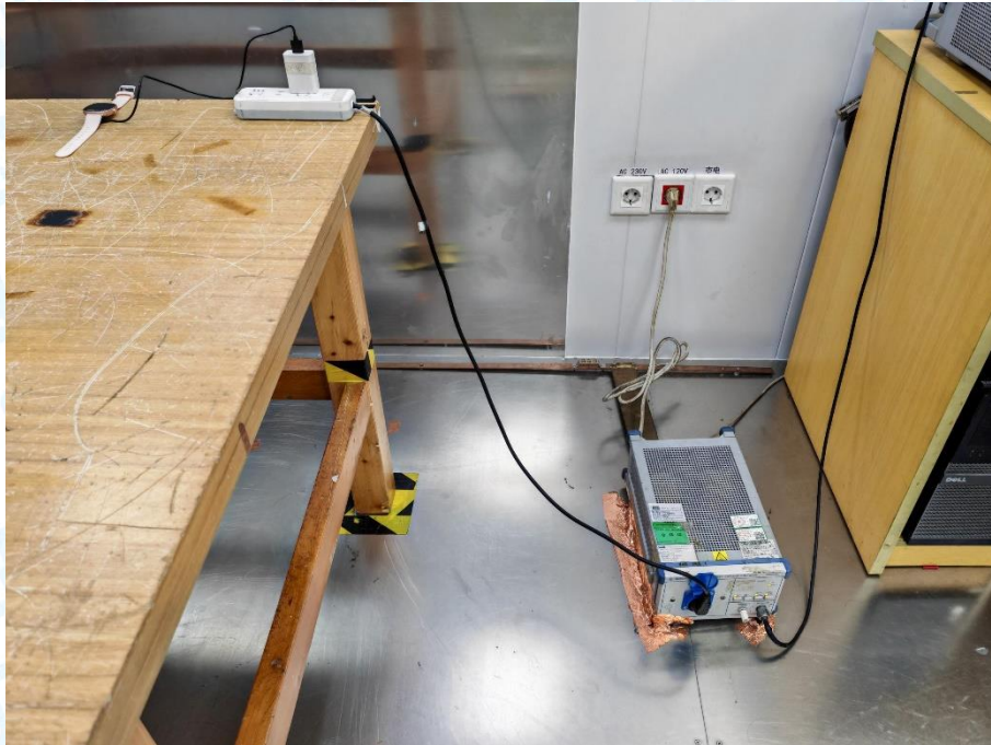
Photo of Setup for Radiated Emission (30MHz~1GHz)
